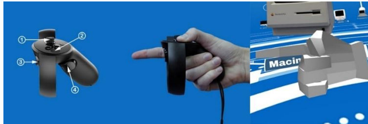
Figure 3.18. Detail of the Oculus Touch controller and the “point” gesture in the virtual museum.
