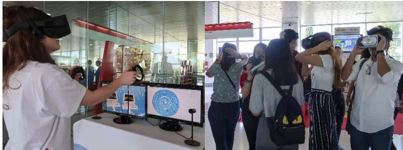
Figure 3.21. The setup of the virtual reality museum study: on the left, a player uses the Oculus interface, while what she sees is displayed on the left screen and the Monitor application is shown on the right screen; on the right, a group of students use the Cardboard interface.
