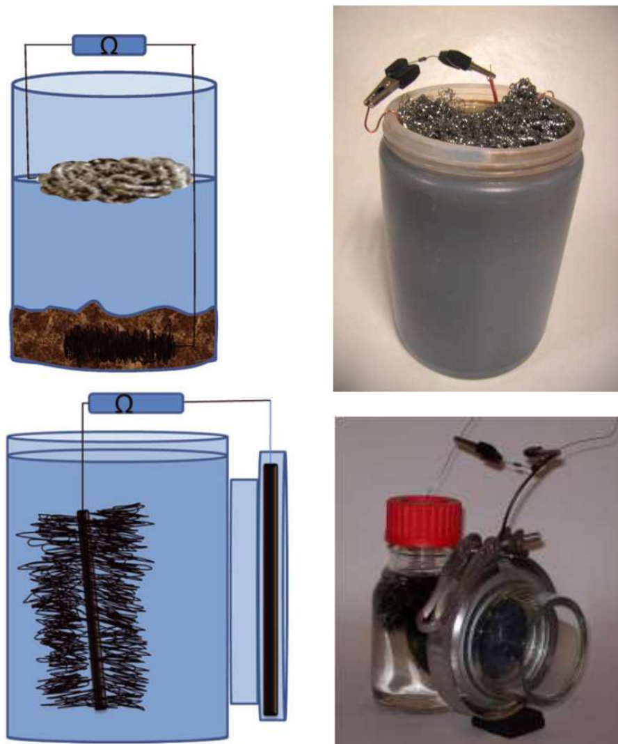
Fig. 4.1. Schematic representations (Left) and pictures (Right) of the Sed-MFC (Top) and the AC-MFC (Bottom)
