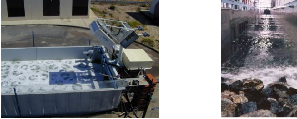
(a) emissivity foam measurements (FROG) and, (b) foam distribution over the waves experiment (UPC facilities).
