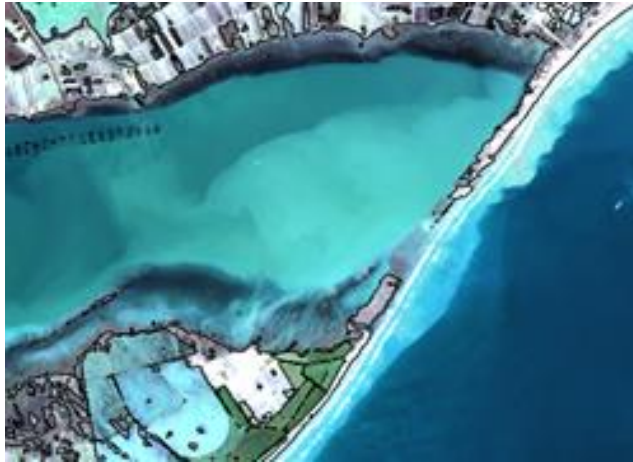
Figure 50. Delineation of emerged land and water surface two weeks after Gloria storm (05.02.20) with the proposed methodology (black line) superposed to the S2 RGB composite.
