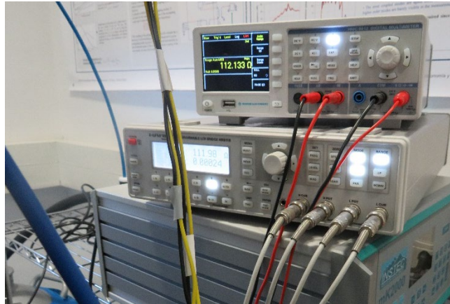
Figure 4. 7. The upper device is the digital multimeter (HMC8012). Then, under the digital multimeter is the LCR-Bridge (HM8118N). Both devices use the 4-wire technique in order to measure the instant resistance of the RTDs.
