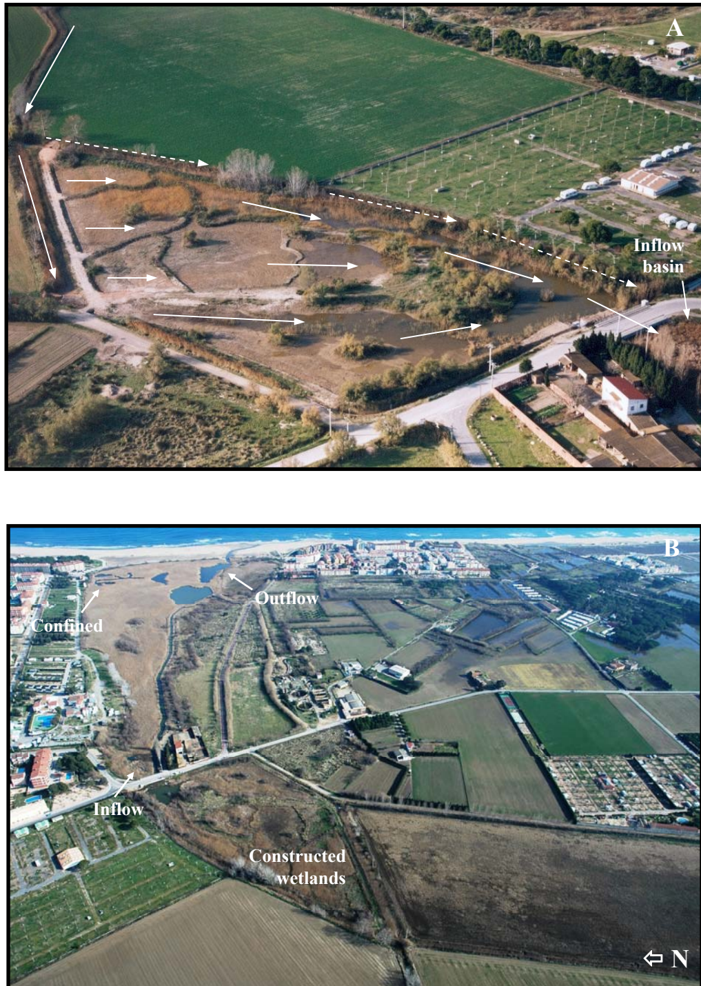
Photo 9. A) Aerial view of the constructed wetlands. The freshwater flux through the treatment system is indicated with solid arrows. The last section of the irrigation channel which fed the lagoon before the construction of wetlands is indicated by dashed arrows. B) Aerial view of the Ter Vell lagoon. The three studied basins (Inflow, Outflow and Confined) and the constructed wetlands are indicated. (Photos by Bon Vent de l'Empordà S.L.).
