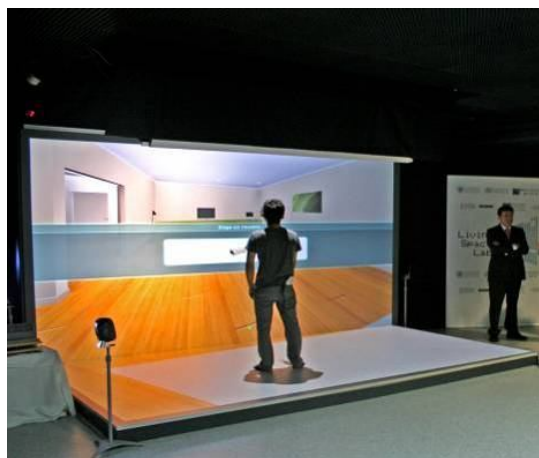
Figura 20. Cave Automatic Virtual Environment (I3BH, 2011)
