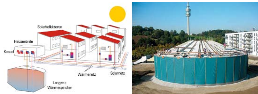
Figure 1.13: (A) Scheme of a solar-assisted district heating plant with seasonal heat storage. (B) Demonstration plant in Munich, 5700 m 3 , 2007 [17]
