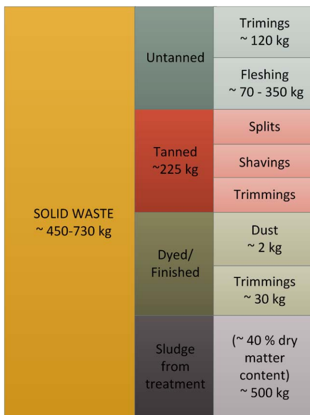
Figure 1.8: Amount of solid waste generated during the manufacturing of leather for bovine salted hides per tonne of raw hide treated
