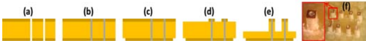
Figure 4.12. Test PCB fabrication process: vias are drilled (a) and filled up with silver paste (b), tracks (c) and pads (d) are patterned on both PCB sides, pillars are created by milling (e) and the final PCB is obtained (f). Inset: detail of one holed pillar.
