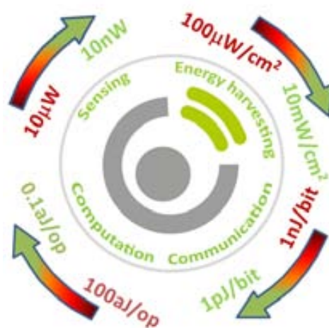
Figure 1.9. Current values of power considered for computation, sensing, communication and energy harvesting and the expected goal values pursued by Guardian Angels UE project.
