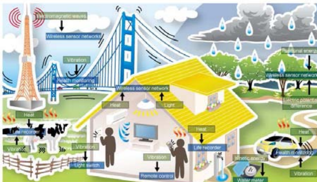
Figure 1.8. Examples of Wireless Sensor Networks and ambient energy sources to power certain applications. (Created by Reiko Kusumoto)
