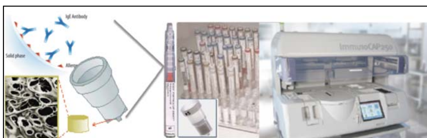
Figure 3.1. Main components of the ImmunoCAP System. The cellulose discs coated with the allergen are placed inside capsules. Capsules are presented inside cylinders (resembling a pen) containing usually 10-12 units. Auto analyzers are able to identify both the sample and the allergen through barcode or sample identification. There are several auto analyzers available depending on the amount of samples that can be processed in one run (e.g., ImmunoCAP 100, 250, 1000, etc.). Adapted from [114].
