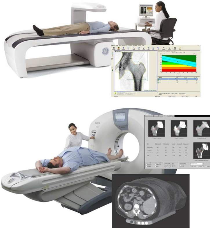
Figure 1.2: A picture of GE Healthcare’s Lunar iDXA scanner (GE Healthcare, Madison, WI, USA) (top) with a screenshot of the software platform, enCORE and GE Healthcare’s Optima CT660 CT System (bottom) with the Mindways calibration phantom and software to perform a QCT analysis (Mindways Software Inc., Austin, TX, United States).
