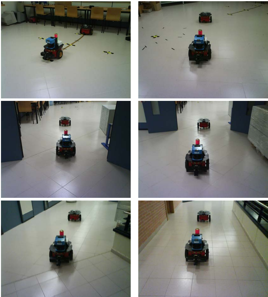
Figure 5.38: Test with two-robot leader-following formation using visual repositioning
