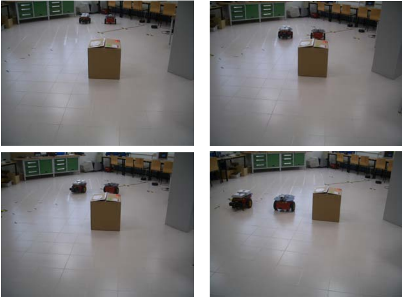
Figure 4.17: Strategy followed in the case that the two robot can pass by the same side
