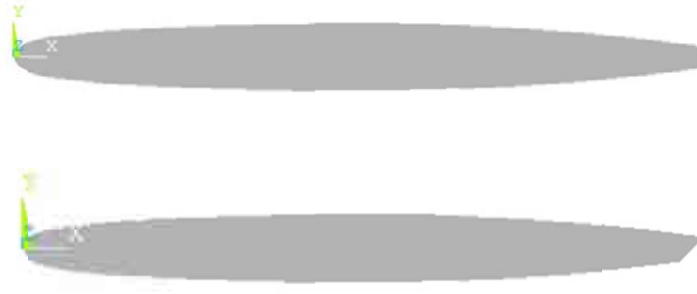
Figure 7.5- 2D views of the different trailing edge solutions adopted. The lower sketch corresponds to the definitive configuration due to its improved performance reducing Von Karman vortices.
