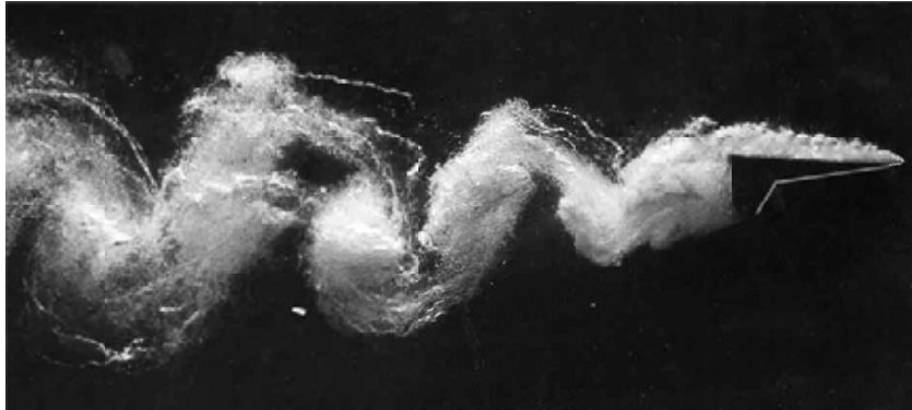
Figure 2.9 - Vortex cavitation (from Brennen 1995).
