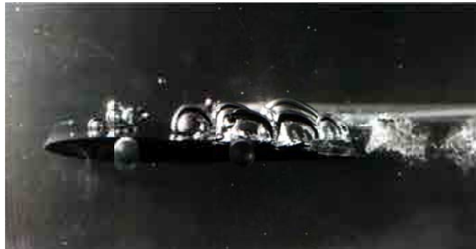
Figure 2.8 - Travelling bubble cavitation (from University of Tokyo).
