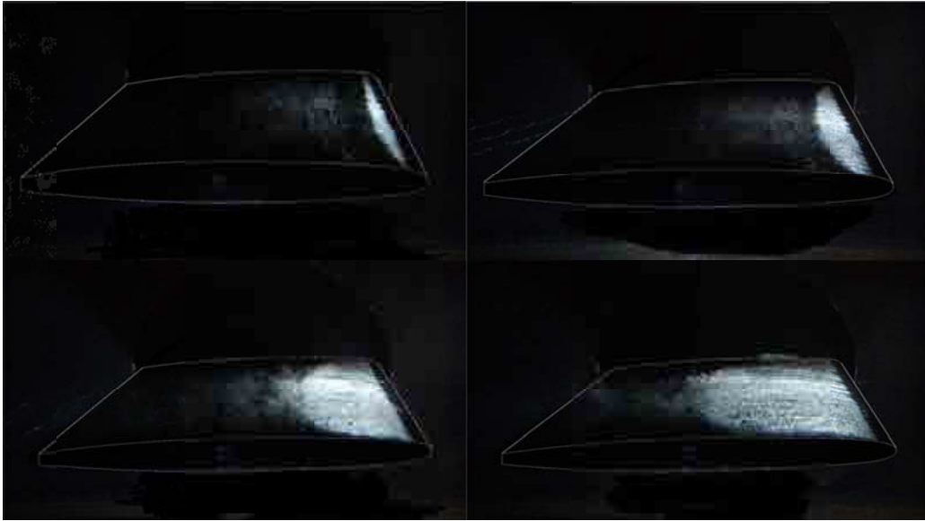
Figure 10.8- A series of pictures representing different cavity lengths at 14 m/s and a 1° incidence angle (above) and a 2° incidence angle (below).
