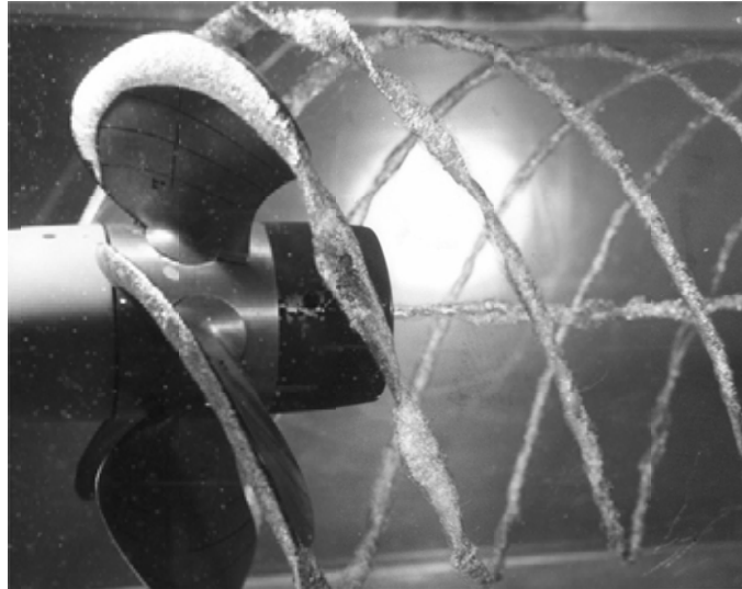
Figure 1.1- Cavitation can take different forms and affect many structures (from Franc and Michel 2004).
