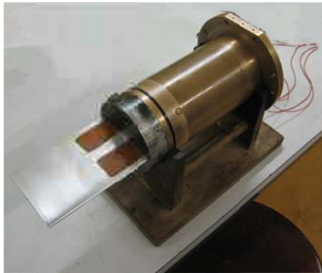
Figure 7.3- Hydrofoil installed on the rigid subsection system.
