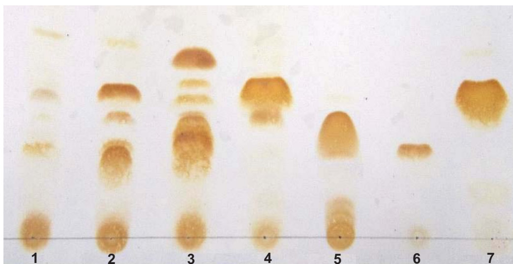
Figure 3. TLC Analysis of Argentinian Amaryllidaceae (BCE). 1: H. jamesonii , 2: P. herbertiana , 3: R. mendocina , 4: Z. filifolia , 5: Galanthamine, 6: Lycorine, 7: Tazettine.
