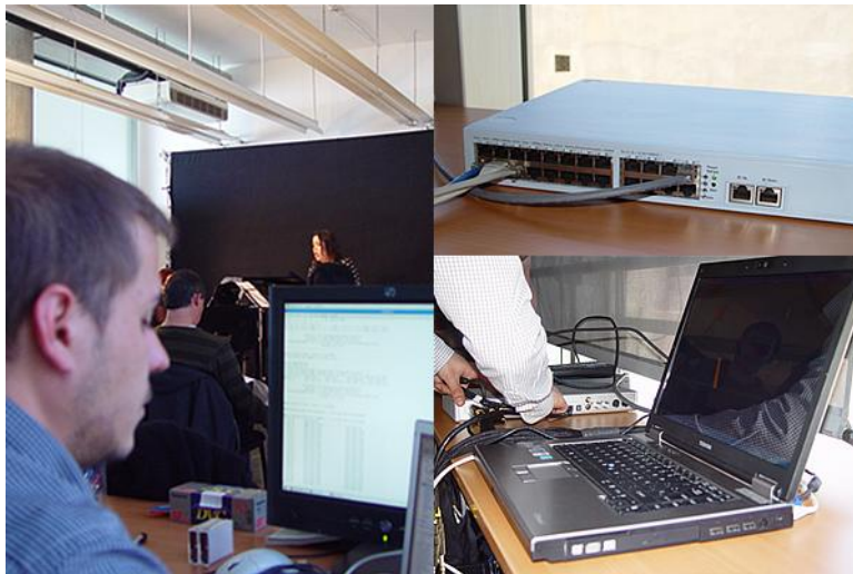
Figure 41. Network transmission computers and digital converters.
