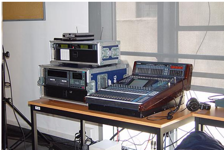
Figure 43. Picture of mixer, recorder and audio equipment.
