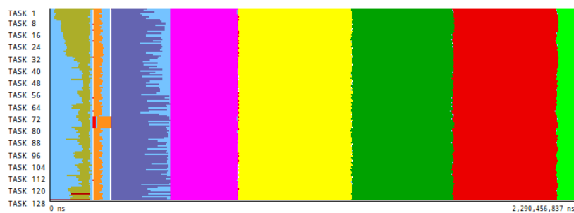
Figure 6.7.: Computation structure detection of Hydro solver, using Aggregative Cluster Refinement algorithm
