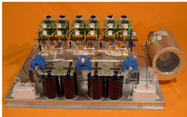
Fig.2.11. NPC converter: (a) general diagram, and (b) converter set up.
