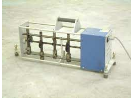
Fig. I.1: Tapping machine. Source: www.sp.se , retrieved on 2013-08-01
