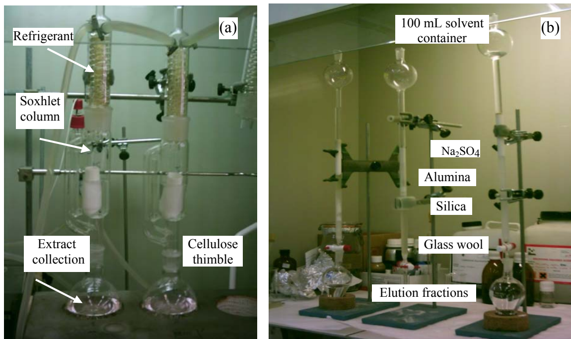
Figure 3.3. (a) Soxhlet extraction and (b) Solid phase extraction.
