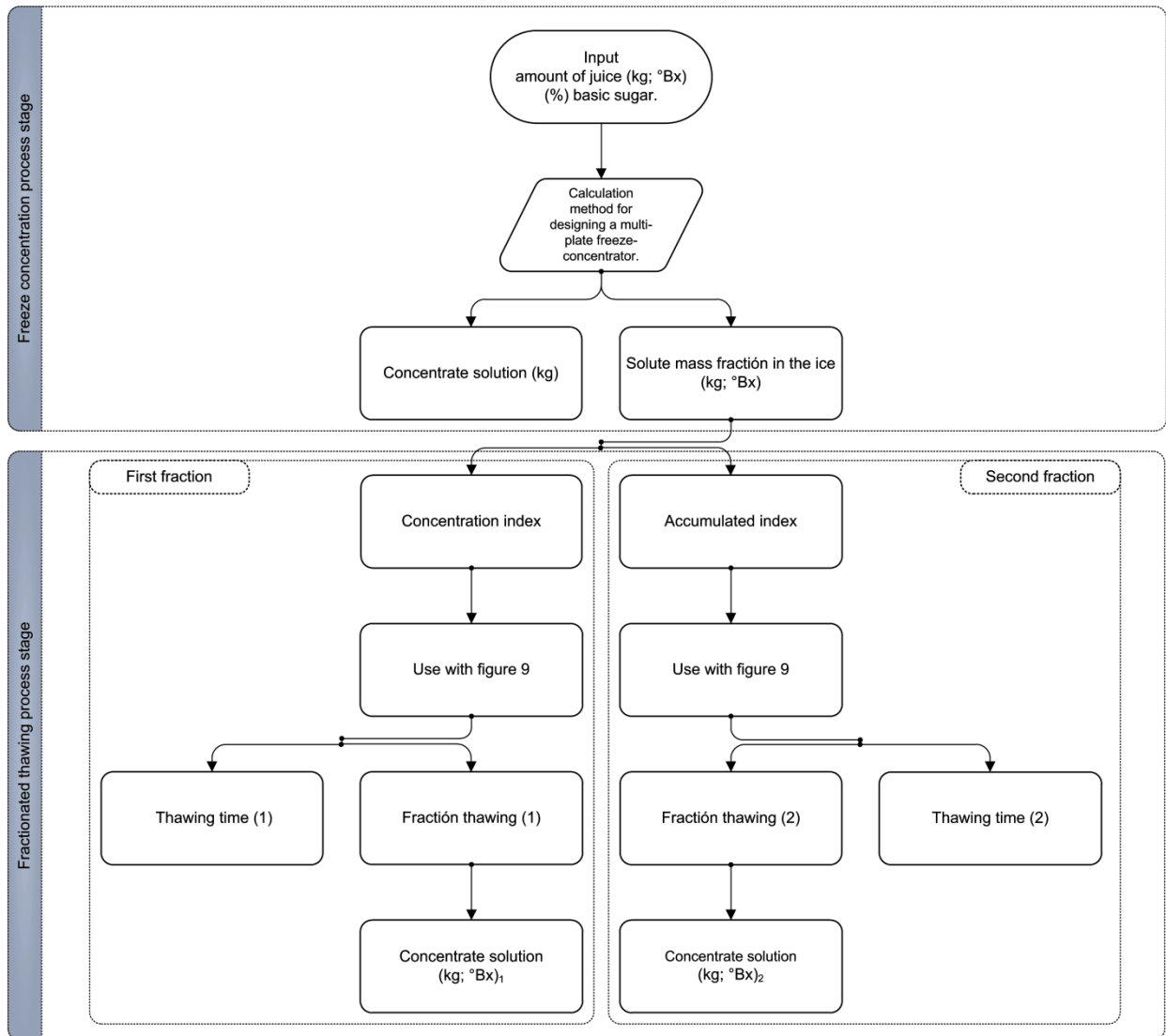
Figure 8. Algorithm for the calculation of one stage of a freeze concentration process.
