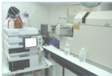
Figure 2.13. Picture of the ICP-MS placed at “Seveis Cientificotècnics UB” used for the analyses.
