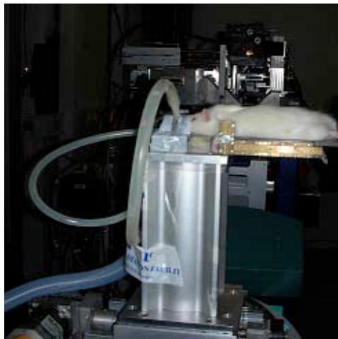
Figure 3.1. Positioning of a rat on the goniometer for MBRT irradiations. Rats were anesthetized in situ with isoflurane inhalation.
