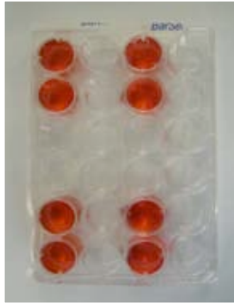
Figure 2.3. Well-seeding distribution. Each plate was covered with an extra-thin and colorless sealing tape enabling the irradiation of the plate vertically.
