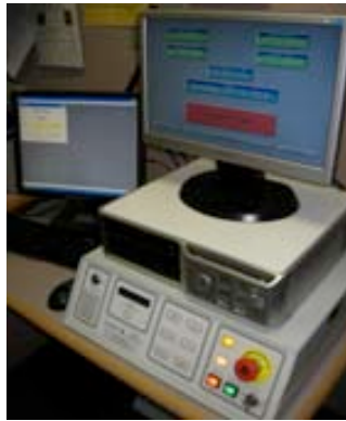
Figure 1.18. Control console placed out of the irradiator's room.
