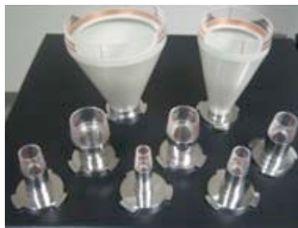
Figure 1.19. Applicators of different diameter-sizes that can be used in the kV irradiators.
