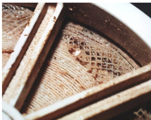
Figure 10. Biofouling causing displacement of feed spacer because of the fouling layer [30].
