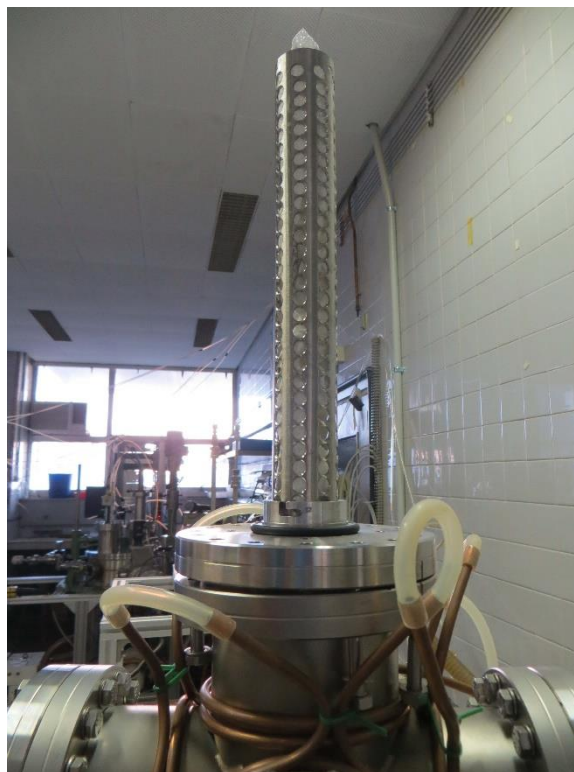
Figure 2.1-7. This stainless steel column was prepared for collecting the particles by making turbulent and capturing them by a paper filter.
