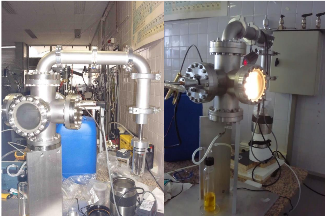
Figure 2.1-6. This is the gas phase reactor based on laminar flow and liquid nitrogen. The collection glass is putted inside a liquid nitrogen box; and so the nanoparticles trapped inside the glass before the gas outlet.
