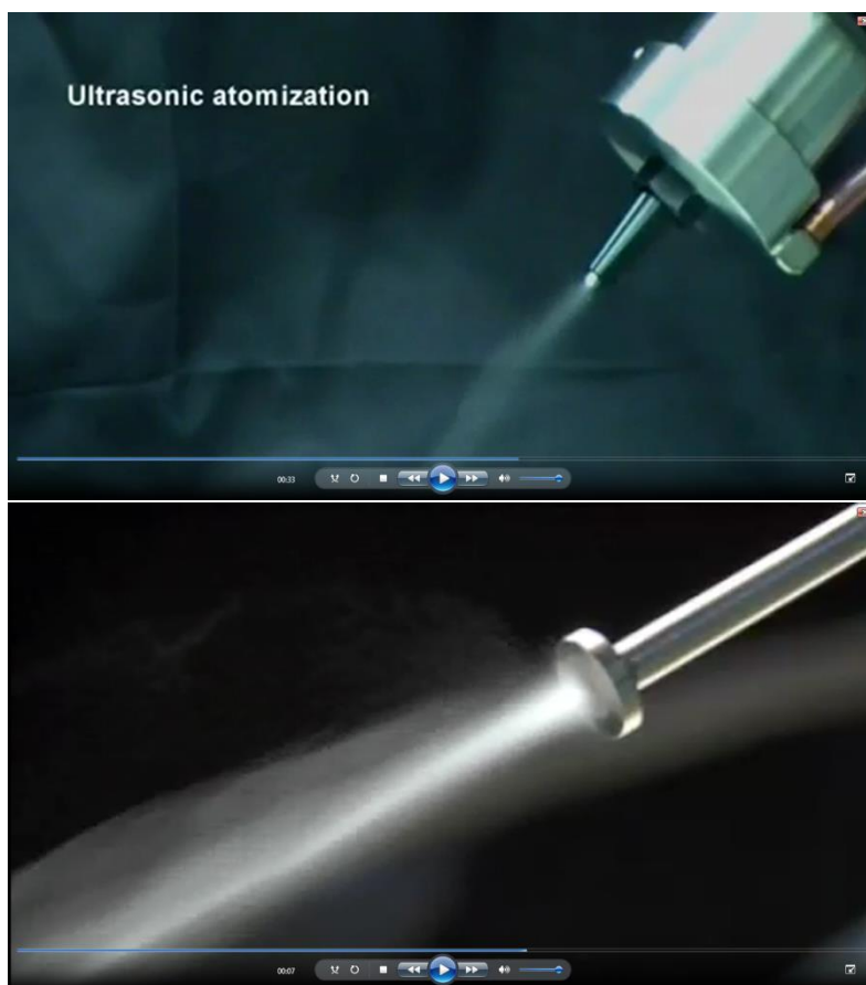
Figure A-1. Ultrasonic atomizer suitable for delivering precursor (Sono-Tek, 2015).
