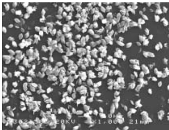
Figure 8a. Calcium oxalate crystals formed: in absence of inhibitors (basically hexagonal calcium oxalate monohydrate crystals can be observed)
