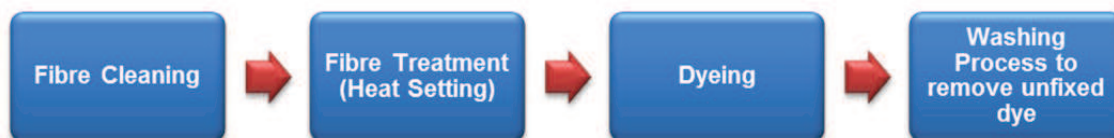
Figure 7.2- Scheme of the dyeing process
