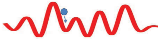
Figure 2.2: The pattern recognition in an associative memory can be visualized by an energy landscape: The local minima illustrate the stored patterns. In the picture, the ball is placed on a slope, which corresponds to a not yet recognized pattern. The arrow indicates the recognition process, in which the ball is pulled into the closest valley.
