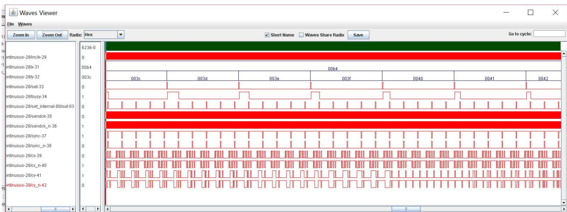
Figure 121 Validation of the XY2-100 serial protocol module with interactive simulation in JHDL
