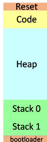
Figure 102 Memory organization for Multithreading support in a NIOS multi-soft-core with 2 processors
