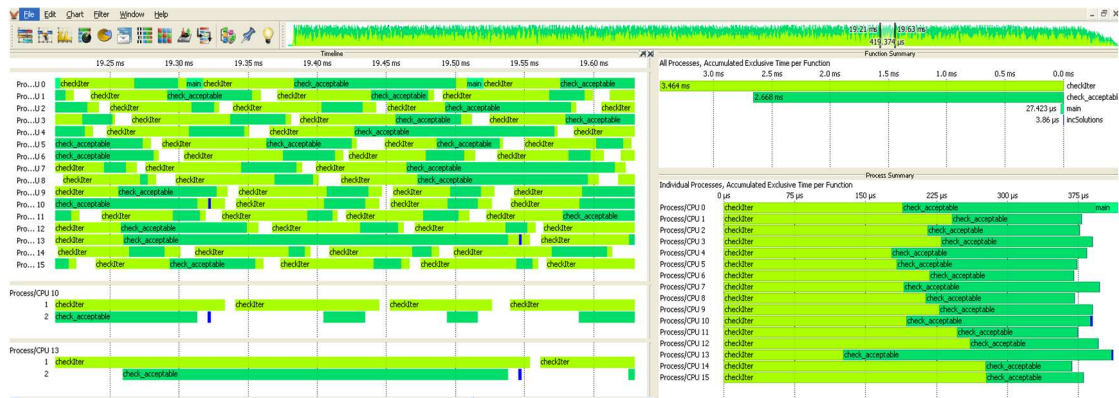
Figure 111 Trace visualization of n -queens application on a 16-core many-core processor virtual platform
