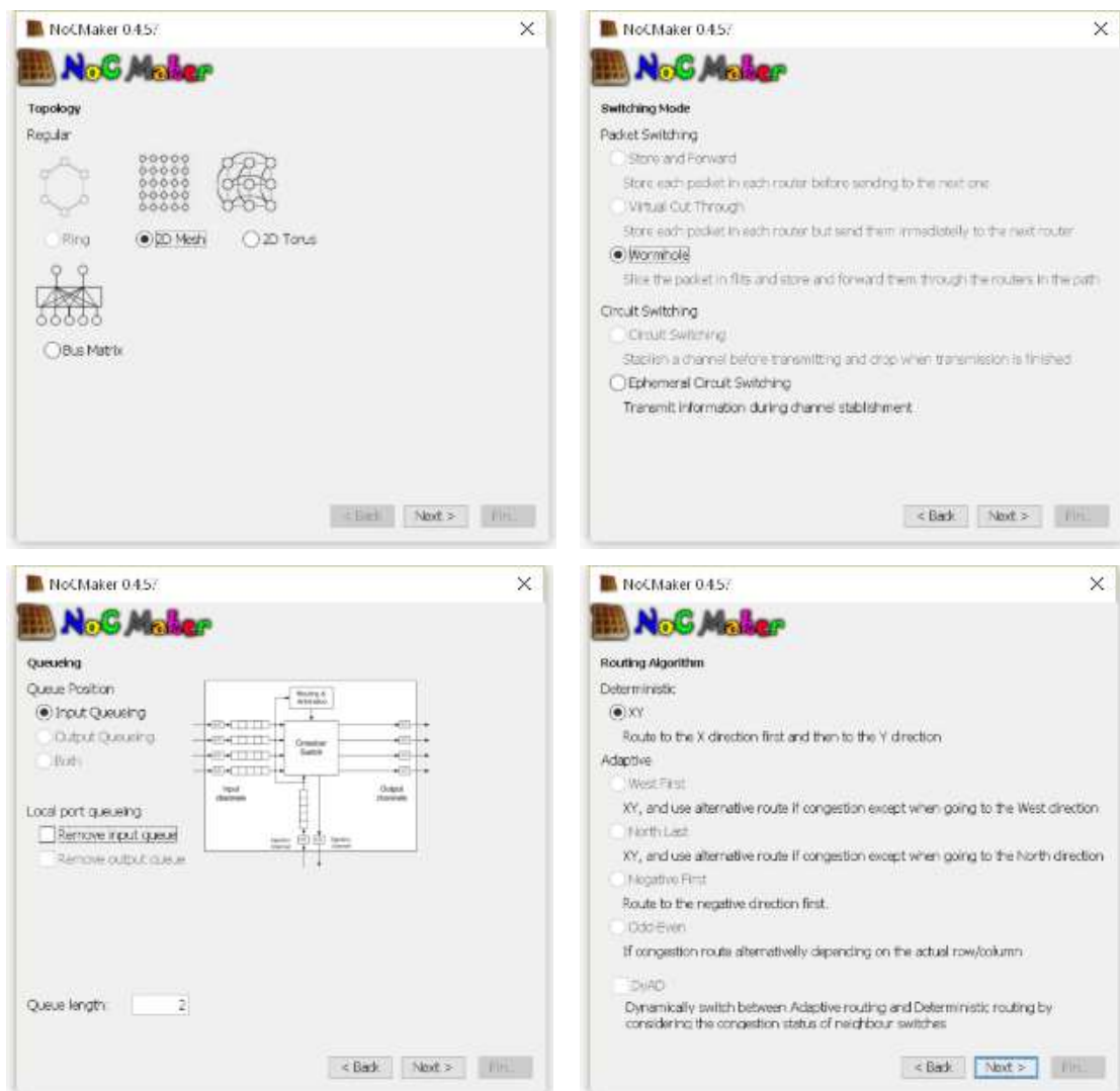
Figure 71 Some of the NoCMaker Wizard screens to create a simple Mesh Network
