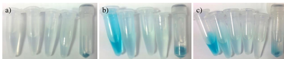
Figure 6.15. MSN-(MB) release a) in MeOH, b) 0.44 M triethylamine in MeOH and c) 0.88 M triethylamine in MeOH.
