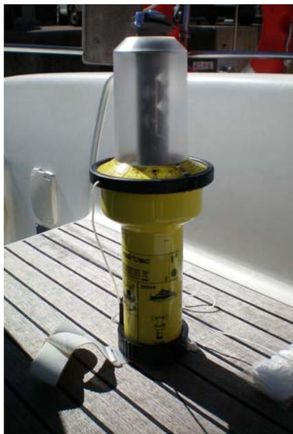
Figure 3. RLB 406 Mhz with GPS. Source: own
