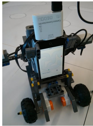
Figure 5.17: Robot used as a haptic in order to solve a maze.
