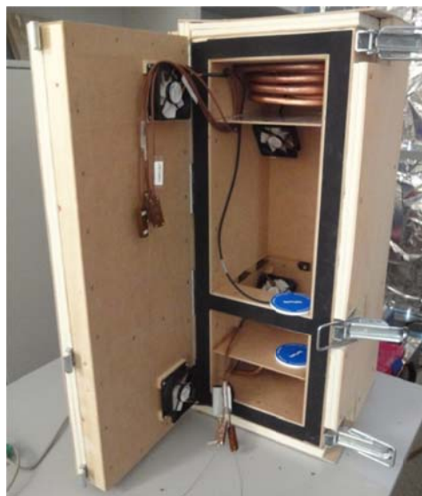
Figure 24. Thermal Behaviour Analyser and examples of data processing
