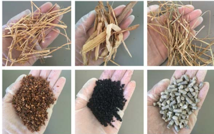
Figure 27. By-products used as additives in adobe bricks.
