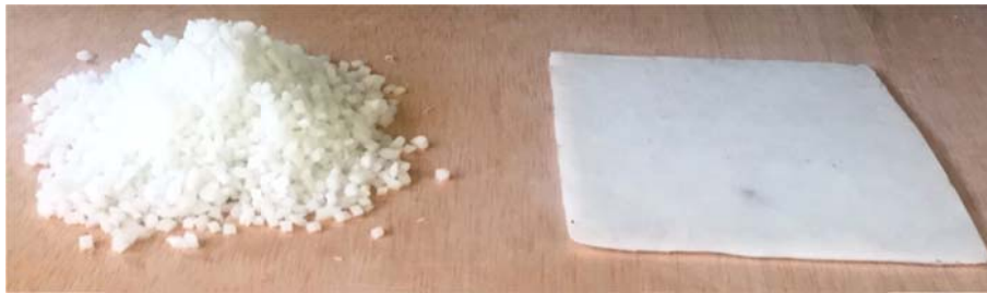
Figure 23. Shape-stabilized fatty-ester PCM: pellets and sheet
