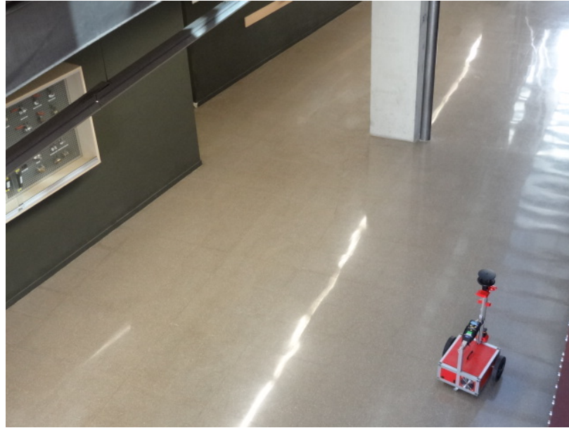
Fig. 5.1. Mobile robot taking ambient measurements while patrolling.
