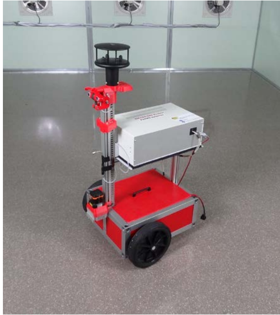
Fig. 7.3. Mobile robot with an IMS as a main chemical sensor device.
