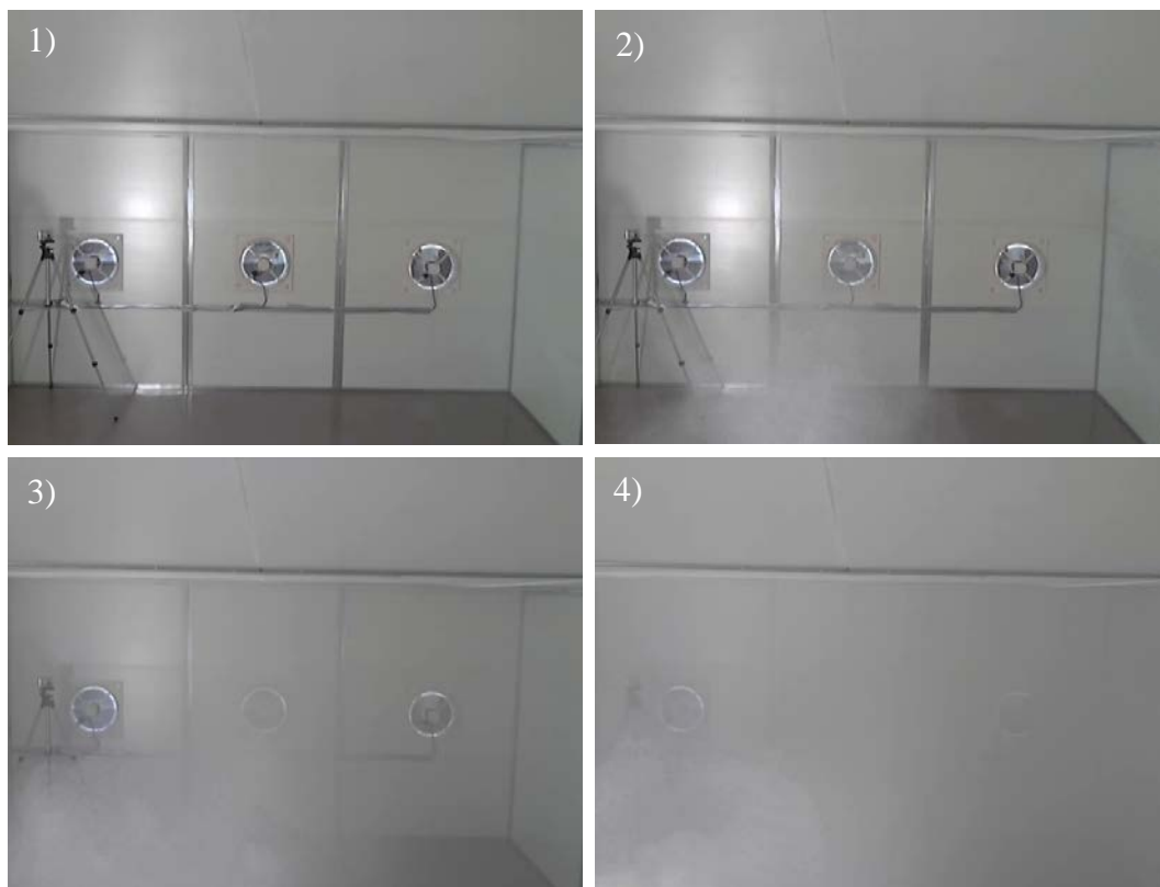
Fig. 6.2. Image captures from the smoke test on the wind tunnel.
