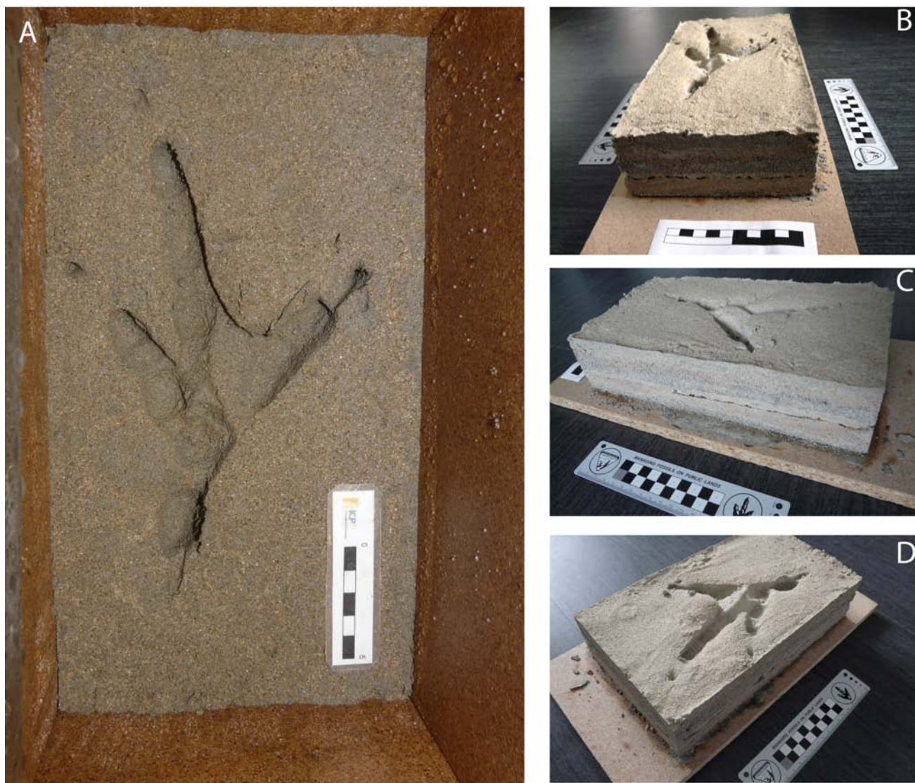
Figure 10.2. A) Track formed after manually indenting the vulture print in a 20% water saturated block of six layers of intercalated medium-grained sands, clays and fine-grained sands. B-D) different views of the six layers package after consolidation of the block of sediments (10-15 days approximately).
