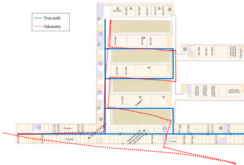
Figure 6.6: Path 1 and odometry obtained with the pocket navigation system.
