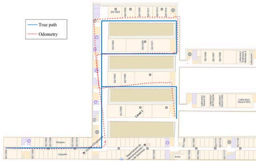
Figure 6.8: Path 3 and odometry obtained with the pocket navigation system.
