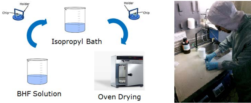
Figure 2.3: Schematic sequence of the wet etching process based on a BHF solution.
