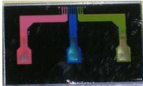
Pictures of a microfluidic network after the fabrication process using silicon technology. (a) Reservoirs and dispensing holes are shown. This side is opened to allow pipette the liquids. (b) Microfluidic channels holding liquid are shown. This side is cover with pyrex.
