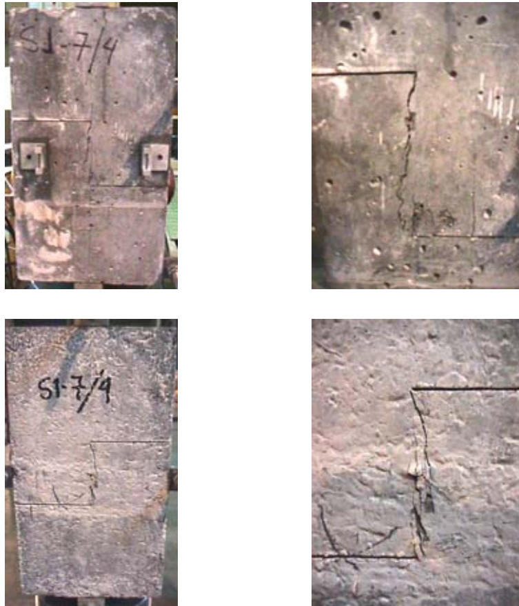
Figure E.30. Modes of Failure. Both sides of the same specimen (whole specimen on the right, failure zone on the left)
