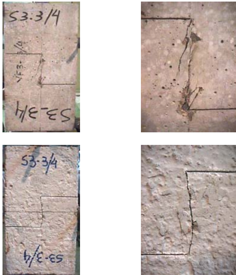
Figure E.17. Modes of Failure. Both sides of the same specimen (whole specimen on the right, failure zone on the left)
