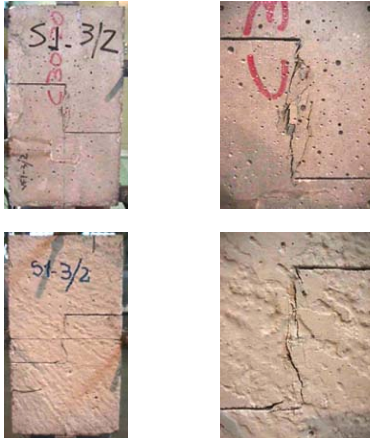
Figure E.7. Modes of Failure. Both sides of the same specimen (whole specimen on the right, failure zone on the left)
