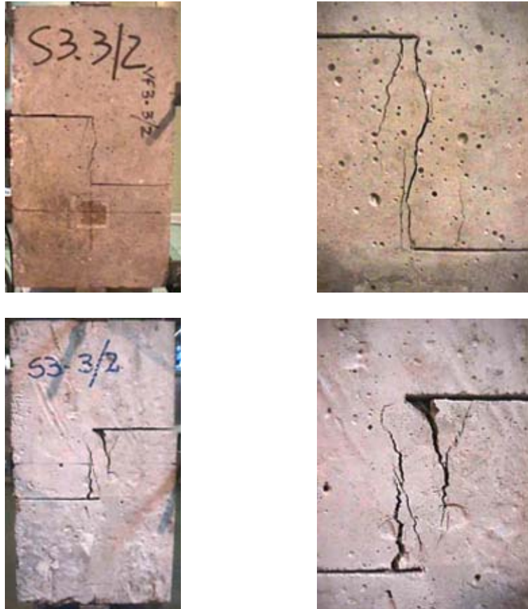
Figure E.11. Modes of Failure. Both sides of the same specimen (whole specimen on the right, failure zone on the left)
