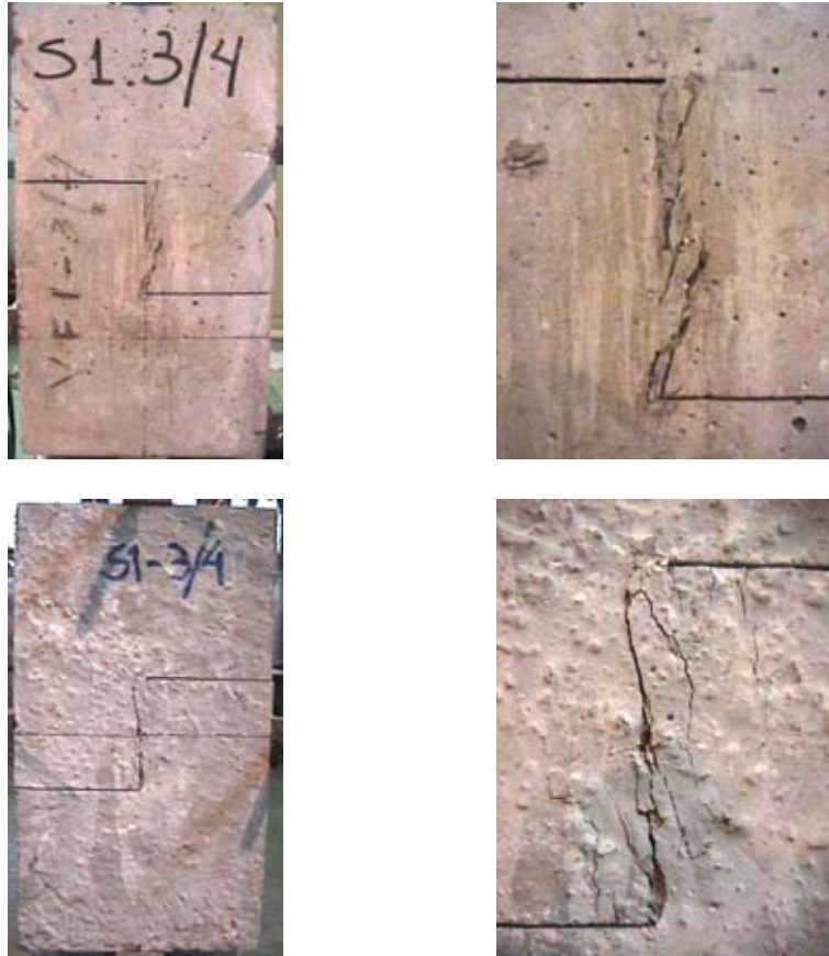
Figure E.13. Modes of Failure. Both sides of the same specimen (whole specimen on the right, failure zone on the left)
