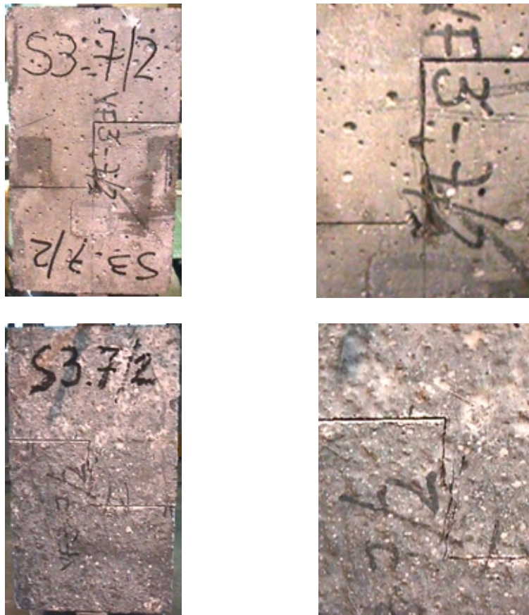
Figure E.28. Modes of Failure. Both sides of the same specimen (whole specimen on the right, failure zone on the left)
