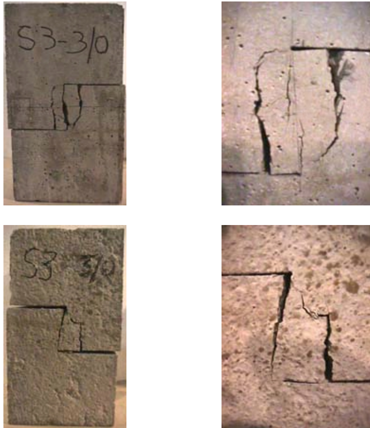
Figure E.5. Modes of Failure. Both sides of the same specimen (whole specimen on the right, failure zone on the left)
