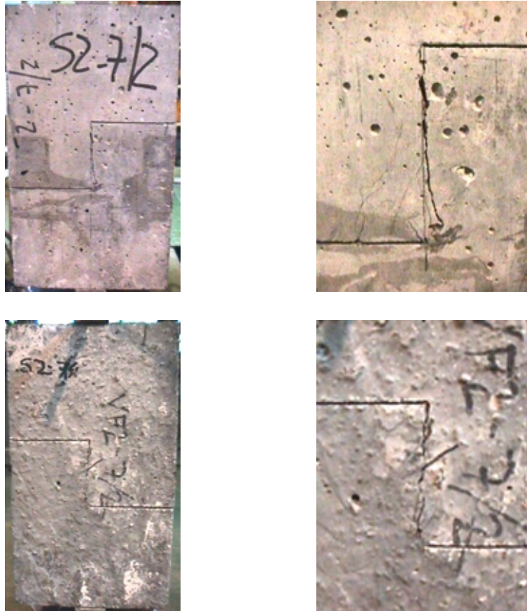
Figure E.26. Modes of Failure. Both sides of the same specimen (whole specimen on the right, failure zone on the left)
