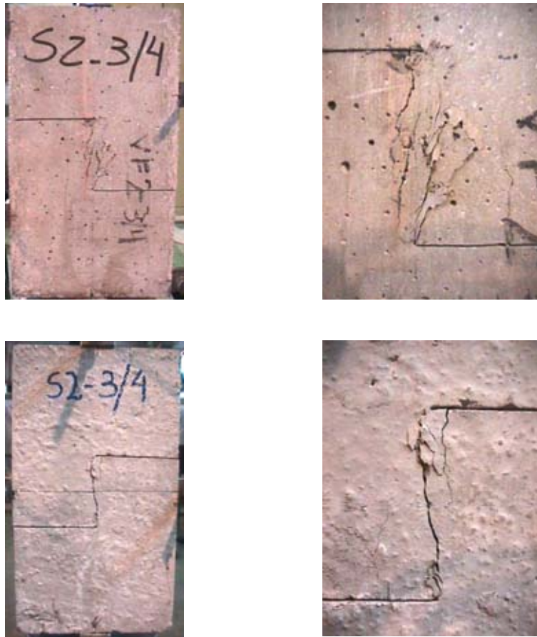
Figure E.15. Modes of Failure. Both sides of the same specimen (whole specimen on the right, failure zone on the left)
