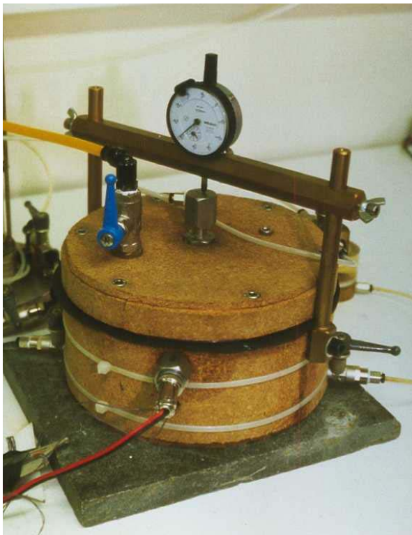
Figure 3.1 Diagram and pictures of the suction and temperature controlled oedometer cell.
