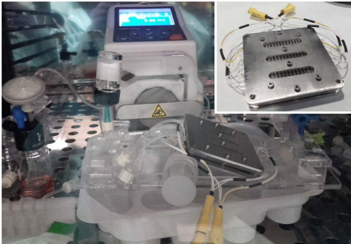
Figure 4-5 Experimental setup including assembly of the perfusion chamber in the top-right corner.
