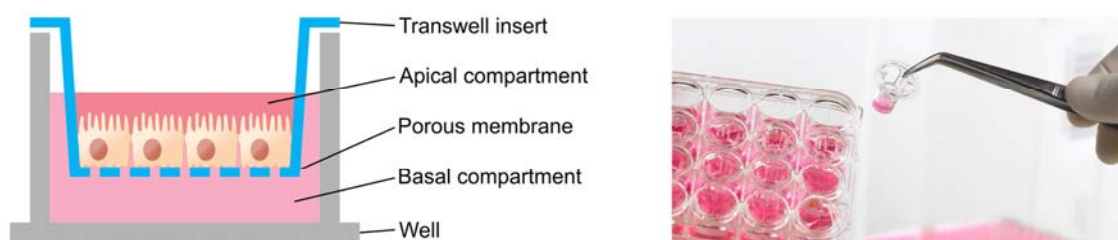
Figure 2-8 Transwell permeable support (Corning Life Science, Corning, NY, US).
