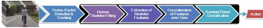
Figure 4.1 – System modules. Framed in black background those which are specific for intention recognition. Note how we are using the same pipeline than for pedestrian intention recognition (see Fig. 2.2)
