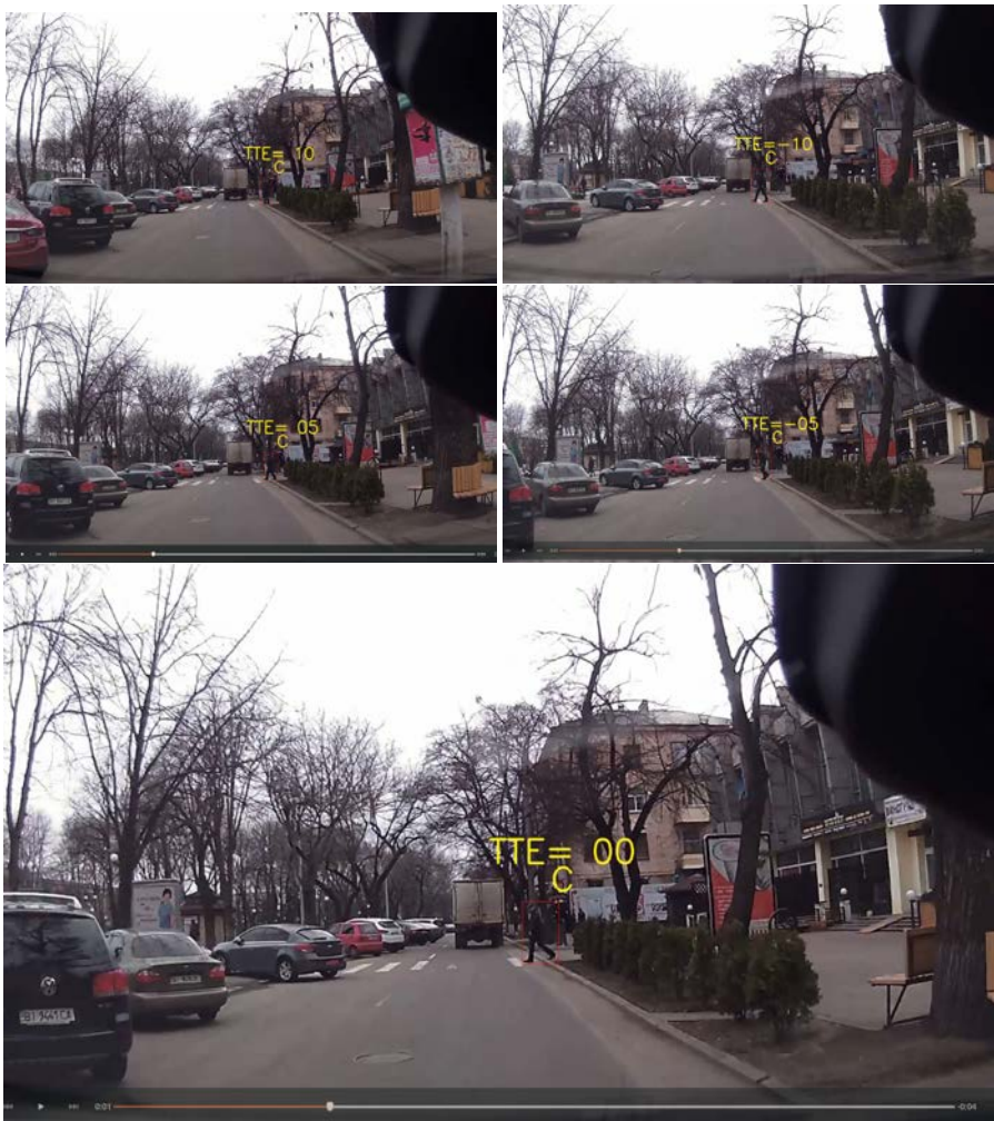
Figure A.14 – Examples of TTE annotation regarding to pedestrian intention recognition in a JAAD sequence. In this case, the pedestrian keeps walking without stopping at the curbside.
