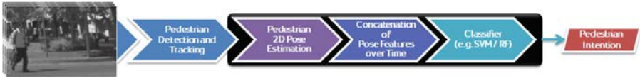
Figure 2.2 – Proposed method. Monocular frames are continuously acquired and processed for detecting and tracking pedestrians. For each tracked pedestrian our proposal consists of: estimating his/her 2D pose by skeleton fitting, computing features from the fitted skeleton; input them to a learned classifier which will output the intention of the pedestrian.
