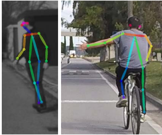
(a) Pedestrian pose estimation by [3]. (b) Cyclist pose estimation by [3].
