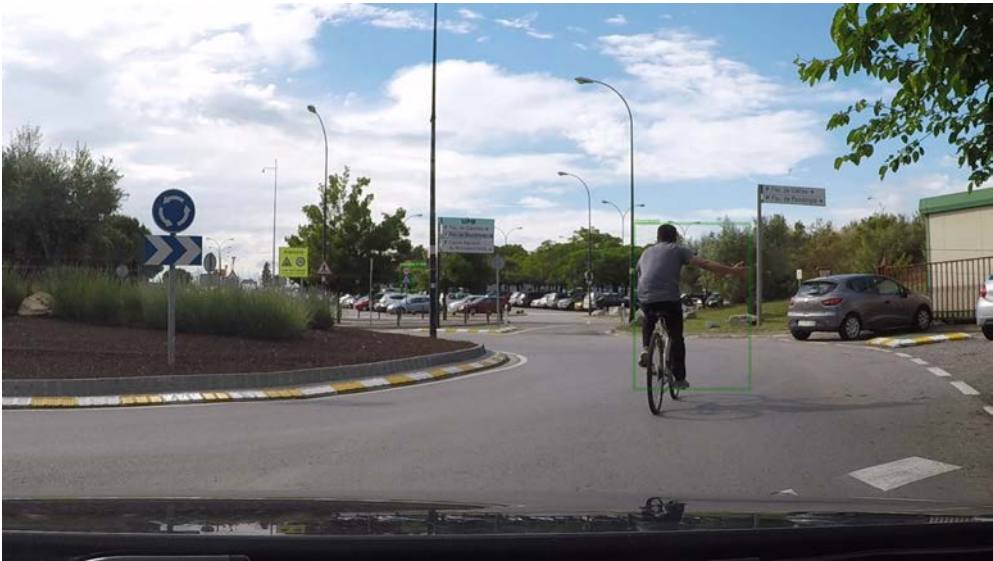
Figure A.6 – Cyclist detection result by using Mask R-CNN [24] and ResNet [26]. Compare the bounding box with Fig. A.4.
