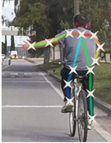
Figure 4.2 – Keypoints used for detecting the intentions of cyclists. 13 keypoints are used to extract 1170 features.
