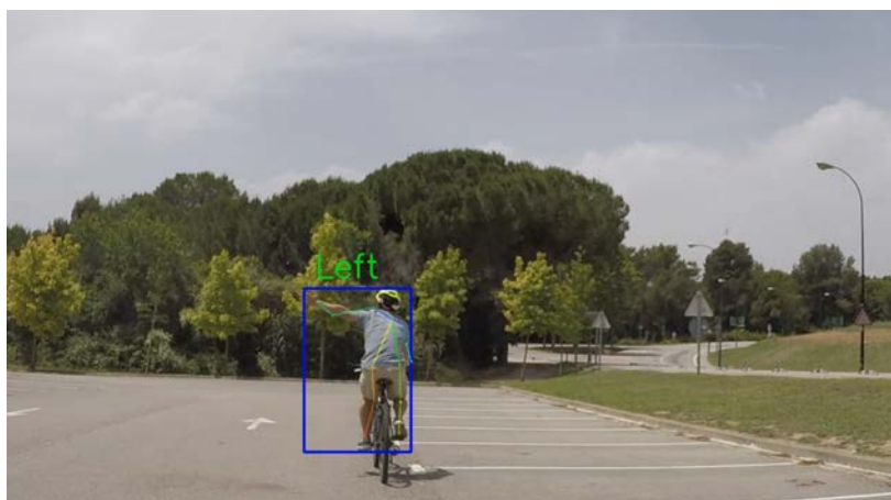
Figure A.22 – Turning left detection with 30 percent of keypoint noise.
