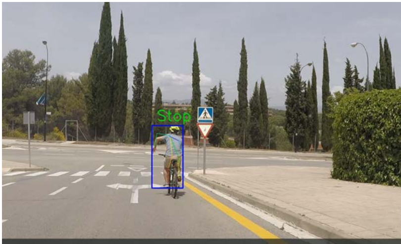
Figure A.25 – Stopping detection with 30 percent of keypoint noise.
