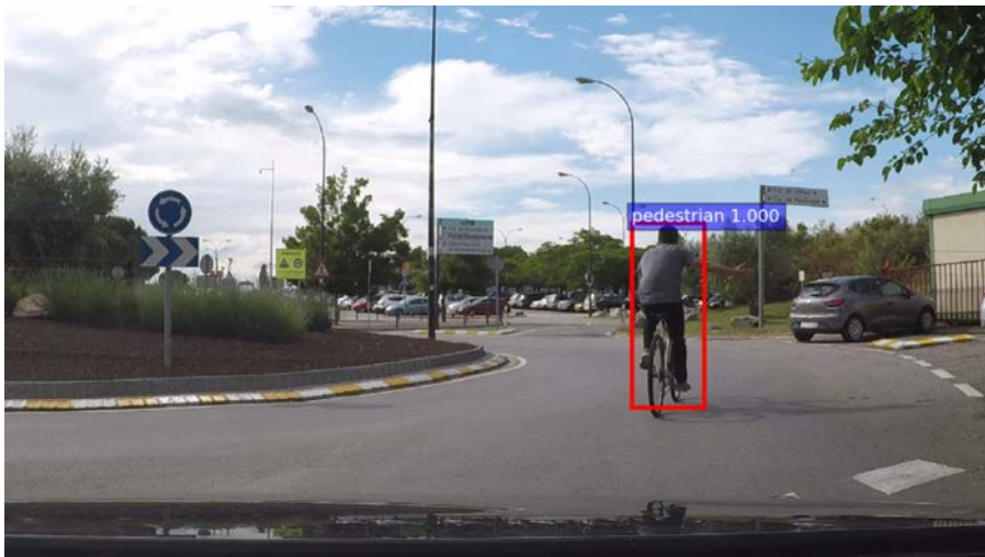
Figure A.4 – Cyclist detection result by using Faster R-CNN [50] and VGG [58].
