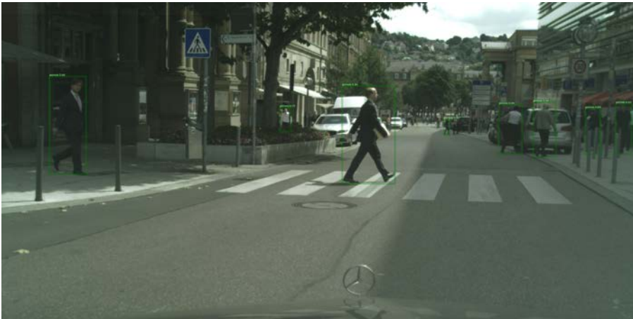
Figure A.8 – Pedestrian detection result by using Mask R-CNN [24] and Resnet [26].
