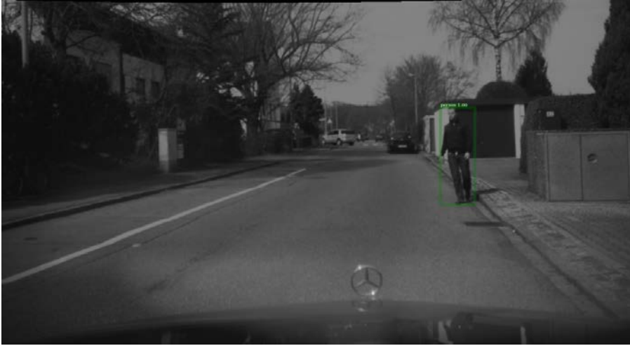
Figure A.7 – Pedestrian detection result by using Mask R-CNN [24] and ResNet [26].
