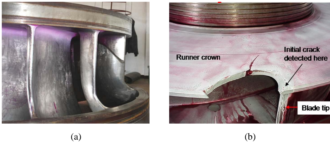
Figure 1-4. (a) Broken Francis runner [13]. (b) Broken Pump-Turbine runner [10].
