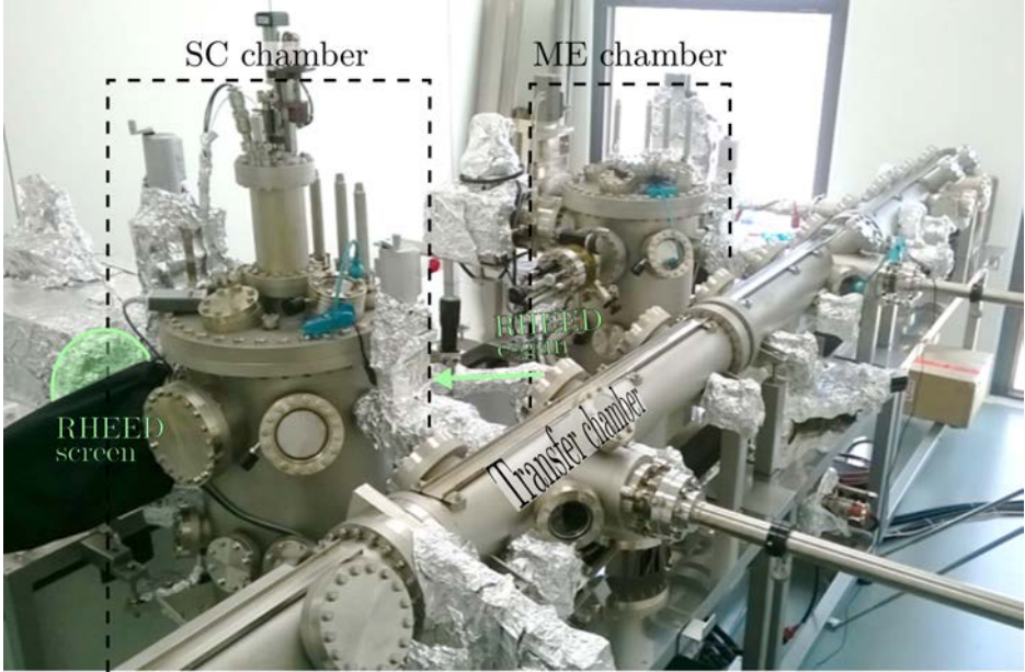
Figure 2.3: The MBE setup at ICN2, formed by two growing chambers, one devoted to the growth of semiconductors (SC) and the other of metals (ME). A transfer chamber enables the UHV connection between them.
