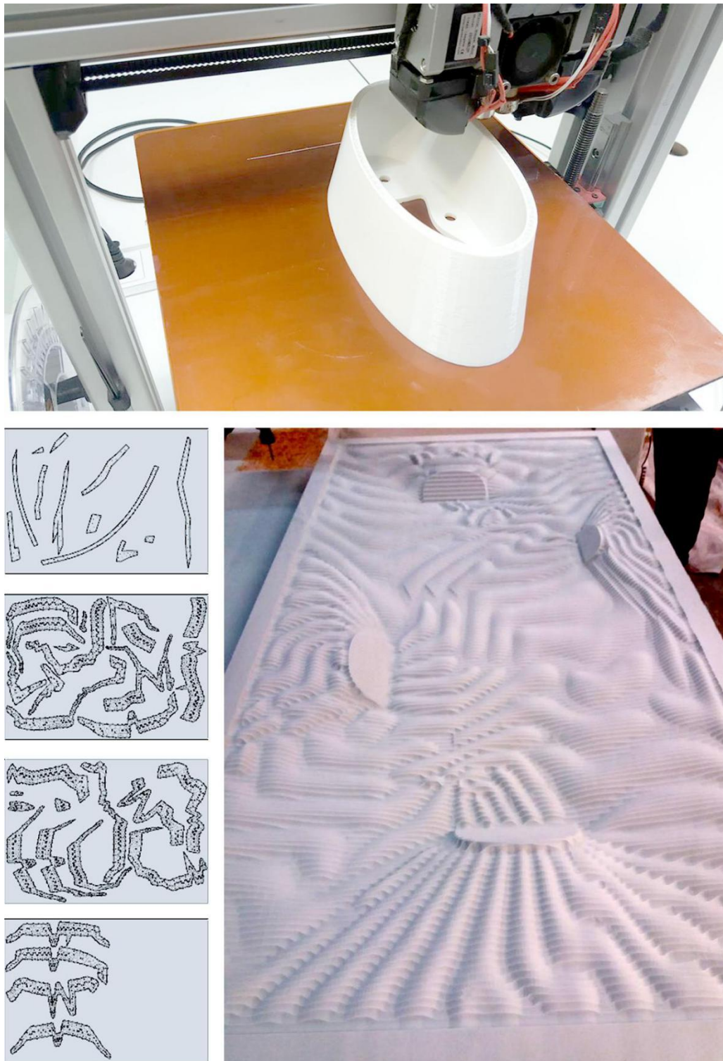
Figure 4. (Bottom right) First milling operation, horizontal roughing, with ball mill (50mm diameter). Stock of 2mm and stepover 50%. (bottom left) nested pieces for laser cutting, (top) 3D printing piece (images by authors)
