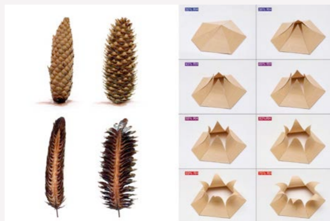
Figure 10. Top: Biological hygroscopic principle found in nature and how it could be applied in the design of passive shape changing wood components. Bottom: Views of open and closed wooden components based on the humidity levels of the environment. Image Courtesy: Institute for Computational Design, 2013
