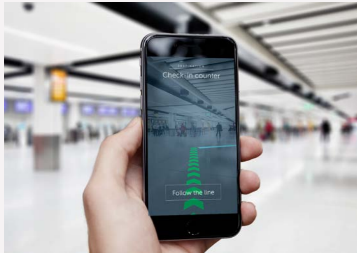
Figure 7. Example of digital indoor navigation tool. View of mobile application for indoor navigation in the London Gatwick Airport. The system is based on the implementation of 2000 beacons (small Bluetooth radio transmitters) that can locate passenger position and provide instructions how to move towards their desired destination. The wayfinding tool, is supported by an augmented reality platform that helps the passenger visualize in physical space the indicated paths. Image Courtesy: PointrLabs http://www.inovateonthenet.net/news/article/uk%27s-gatwick-airport-installs-navigation-beacons-for-augmented-reality-wayfinding
