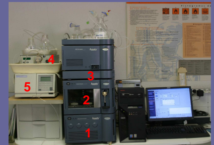
Figura 1. Sistema UPLC (acquity, Waters). 1: bomba binaria; 2: inyector automático; 3: horno con columna UPLC BEH C18; 4: bomba post-columna; 5: detector fluorescencia
