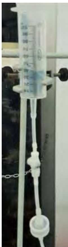
Figure II-6. Gravity method used for the introduction of microplastics aqueous dispersion into the COA device system
