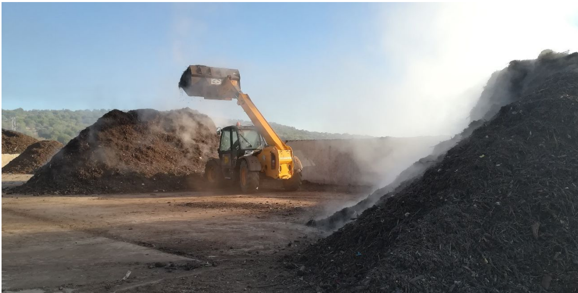
Figure 3.2. Curing or maturation piles and front loader tractor used for mixing.
