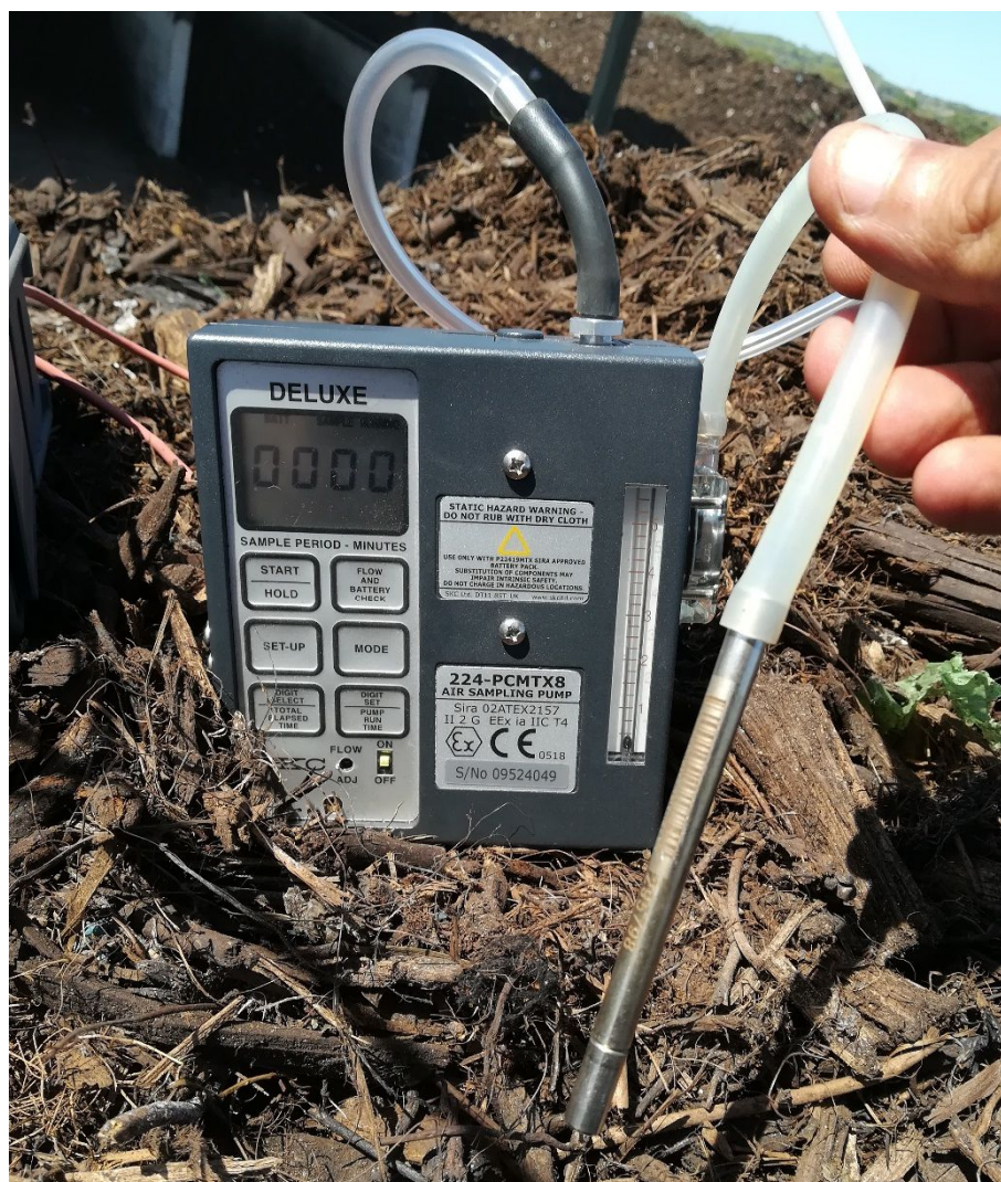
Figure 3.7. Adsorption tubes and automatic gas sampling pump used to obtain gaseous samples for VOCs characterization.
