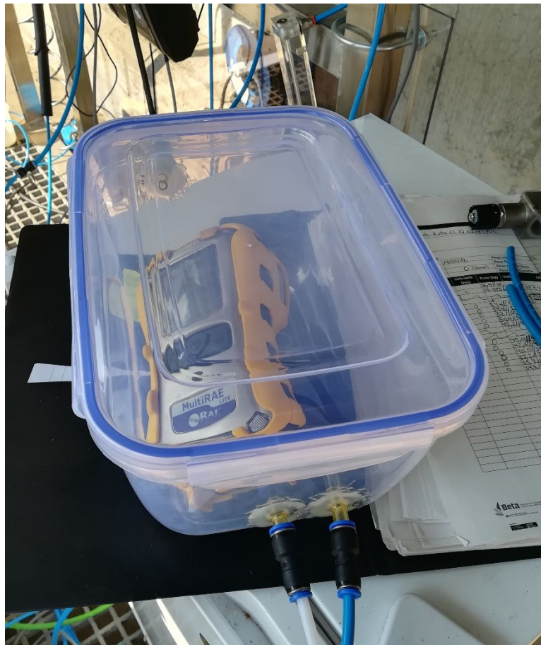
Figure 3.10. MultiRAE Lite portable analyser installed in the hermetic box for tVOCs, \text{NH}_3 and \text{H}_2\text{S} measurement.
