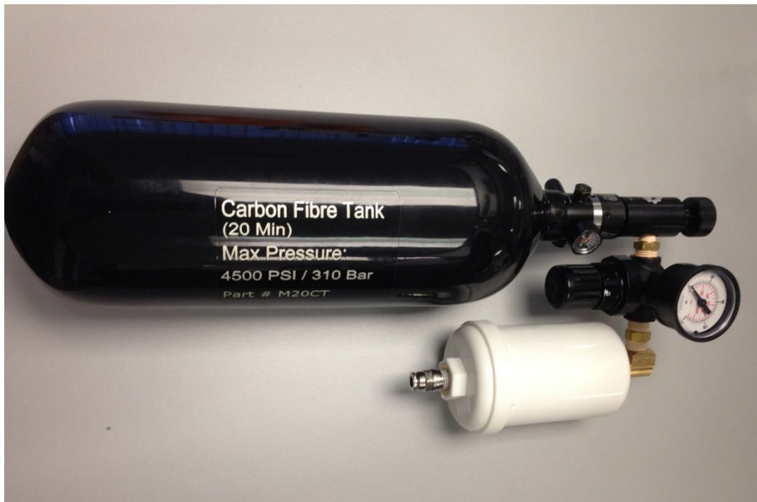
Figure 3.12. Clean air supply-tank, pressure reducer and activated carbon filter of the Scentroid SM-100 portable field dynamic olfactometer.
