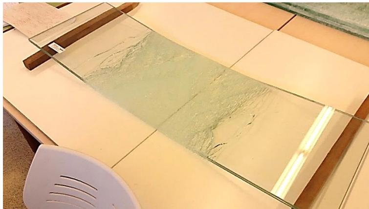
Figure 22. Broken laminated glass specimen after the three-point bending test.
