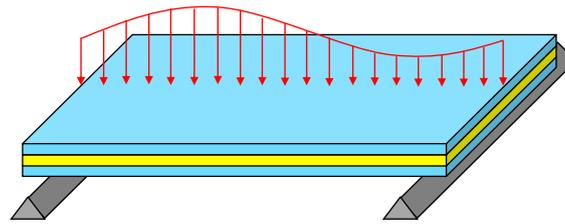
(a) Laminated glass plate (out-of-plane load)
