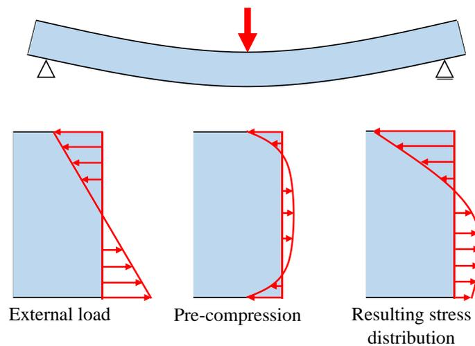
Figure 4. Stress distribution in the cross section of a heat-strengthened glass plate subjected to bending.
