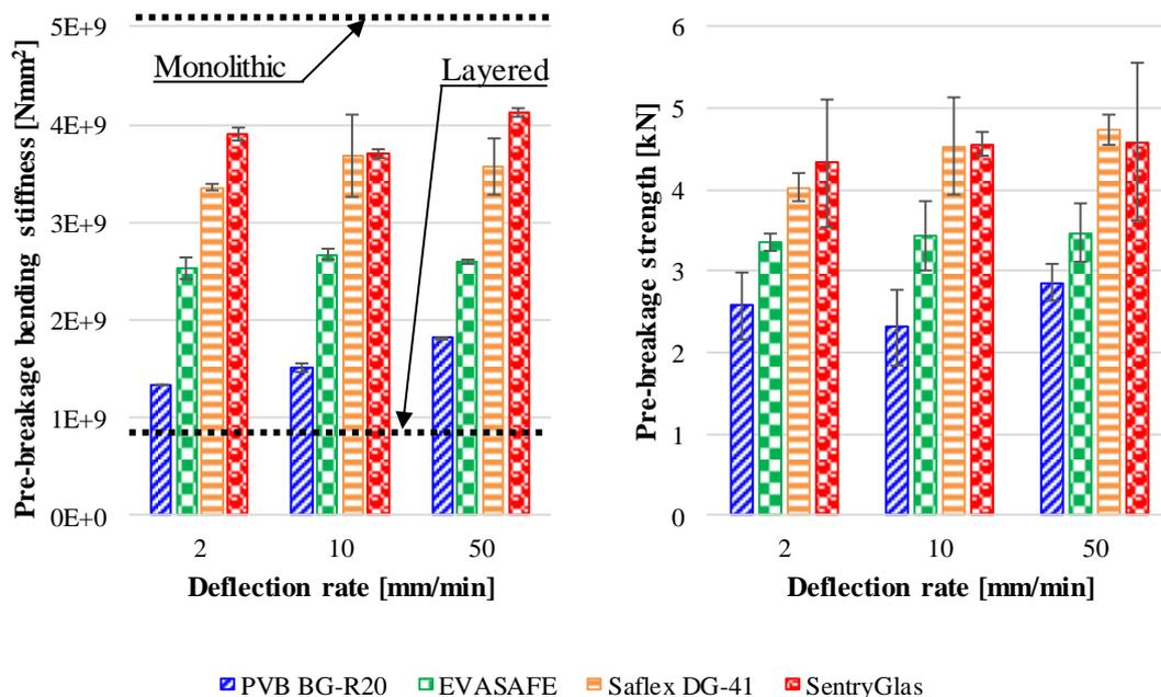
Figure 29. Column diagrams comparing the pre-breakage bending stiffness, calculated using the ESC, and the maximum load of the specimens with different interlayers.
