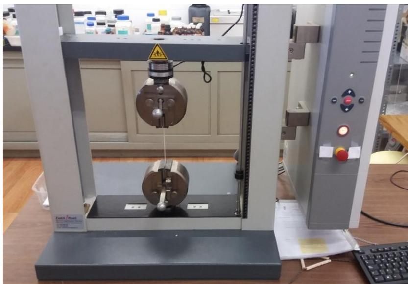
Figure 19. Tensile test on a polymeric film.
