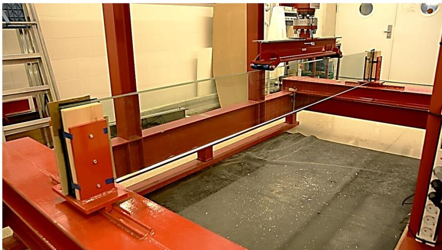
Figure 23. Four-point bending test on laminated glass beams.
