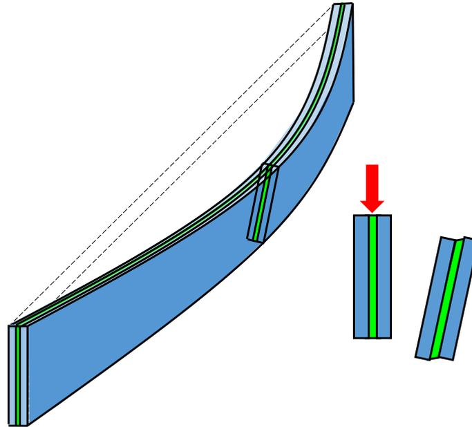
Figure 9. Lateral torsional buckling of a laminated glass beam.
