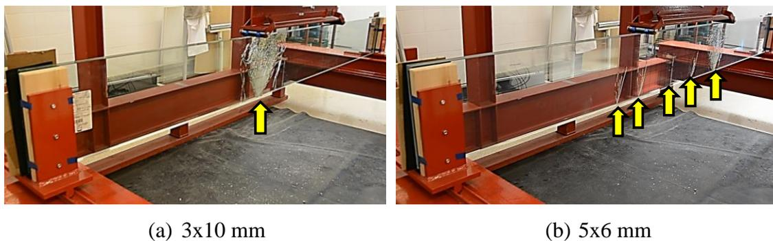
Figure 32. Comparison between the breakage mode of a laminated glass beam with 3 layers of 10 mm and another with 5 layers of 6 mm.
