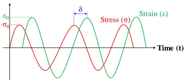
Figure 12. Mechanical response of a viscoelastic material under an oscillatory load.
