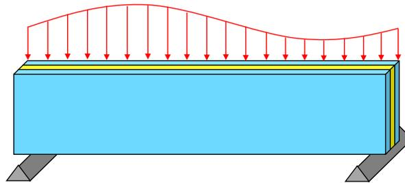
(b) Laminated glass beam (in-plane load)
