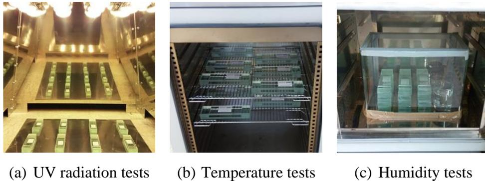
Figure 28. Setup of the different ageing tests.
