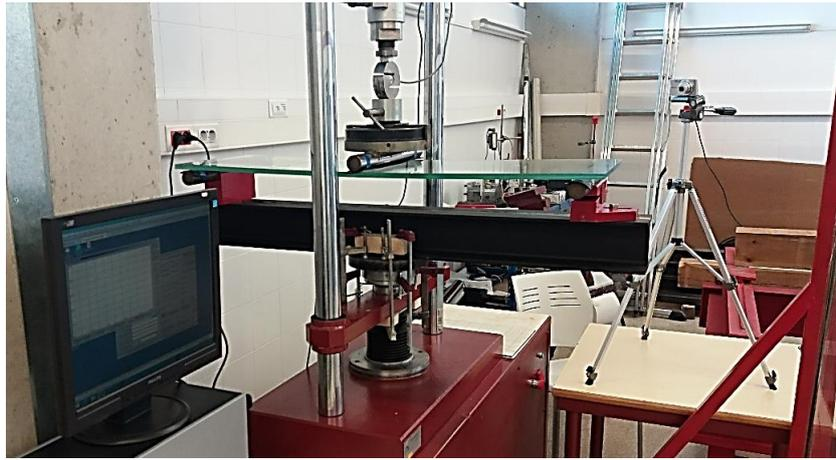
Figure 21. Three-point bending test on a laminated glass plate.
