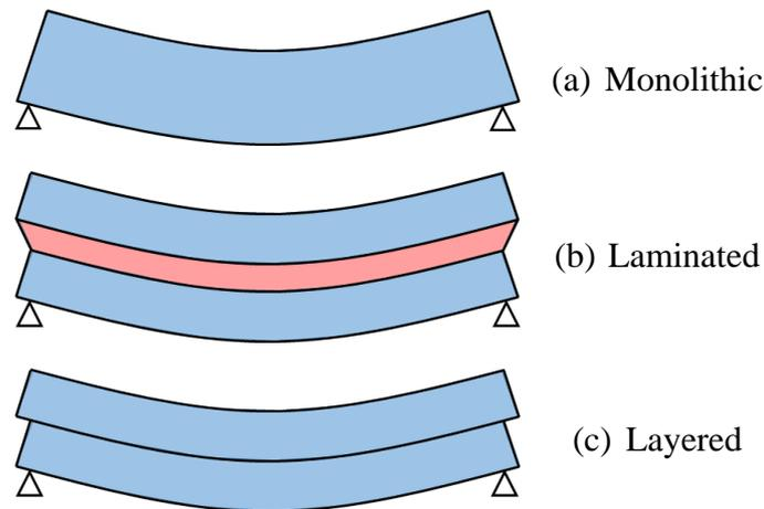
Figure 8. Comparison between the bending of a monolithic, a laminated, and a layered element.
