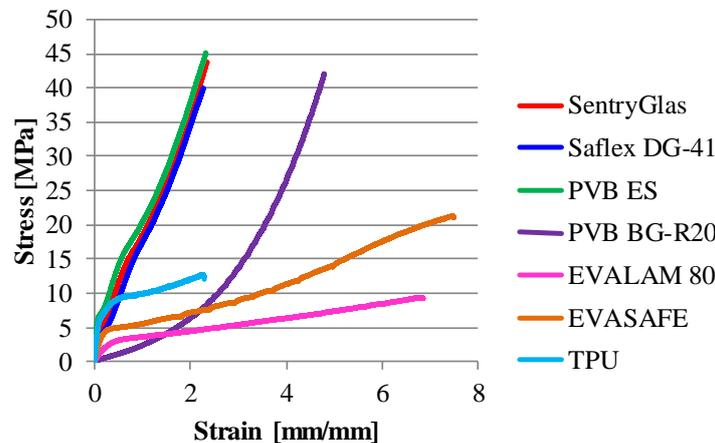
Figure 26. Stress-strain diagram with the results of the tensile tests for all the interlayer materials at the same strain rate (10 mm/min).
