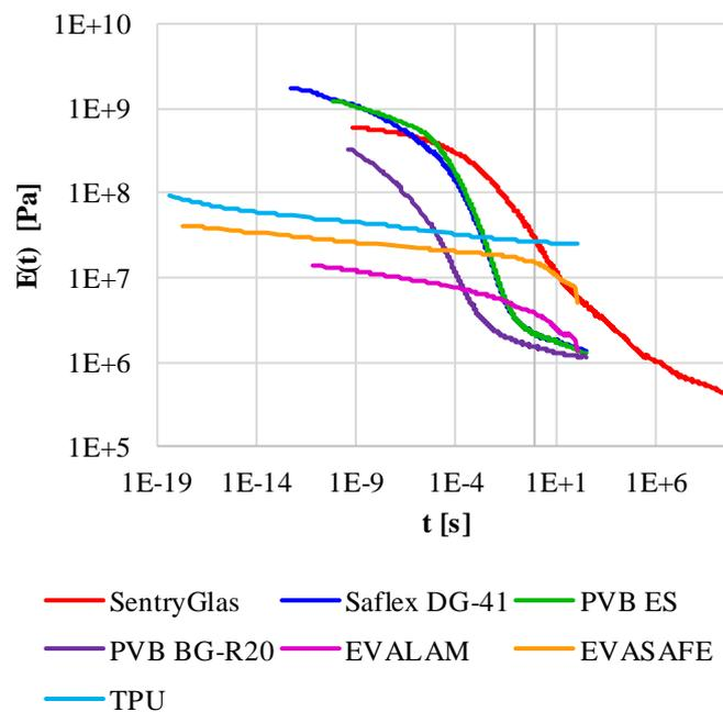
Figure 27. Relaxation master curves of seven different polymeric interlayers obtained from DMA tests.
