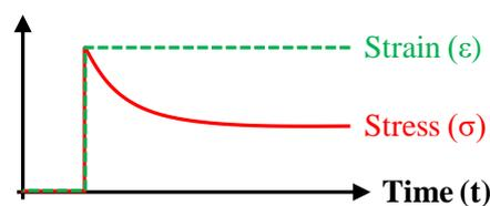
Figure 11. Stress relaxation experienced by a viscoelastic material under a constant strain in a stationary test.
