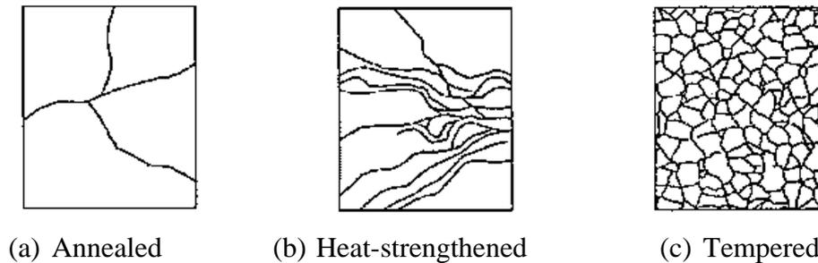
Figure 5. Crack pattern of (a) annealed glass, (b) heat-strengthened glass, and (c) thermally toughened or tempered glass. Retrieved from [14].
