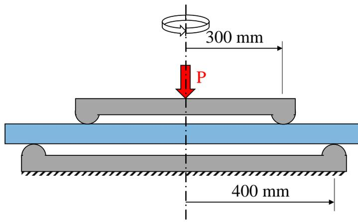
Figure 13. Coaxial double ring test proposed by the standard ISO 1288-2 [38].
