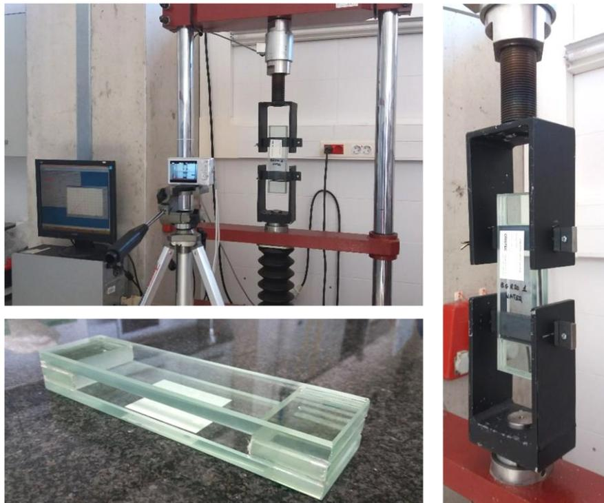
Figure 20. Double-lap shear test.
