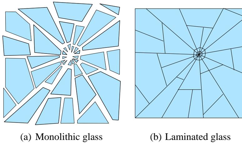
Figure 6. Sketch of the breakage of monolithic glass and laminated glass.
