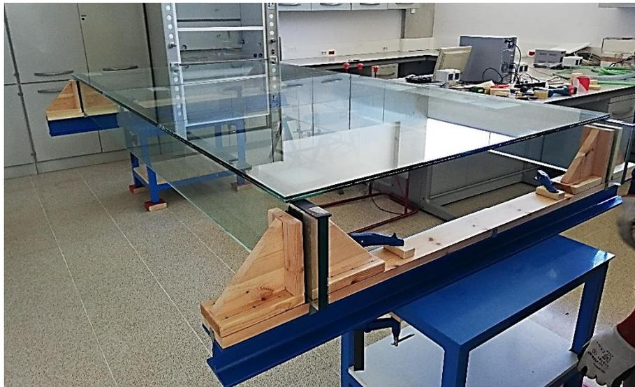
Figure 24. Laminated glass slab placed on a metallic structure with wooden lateral restraints.
