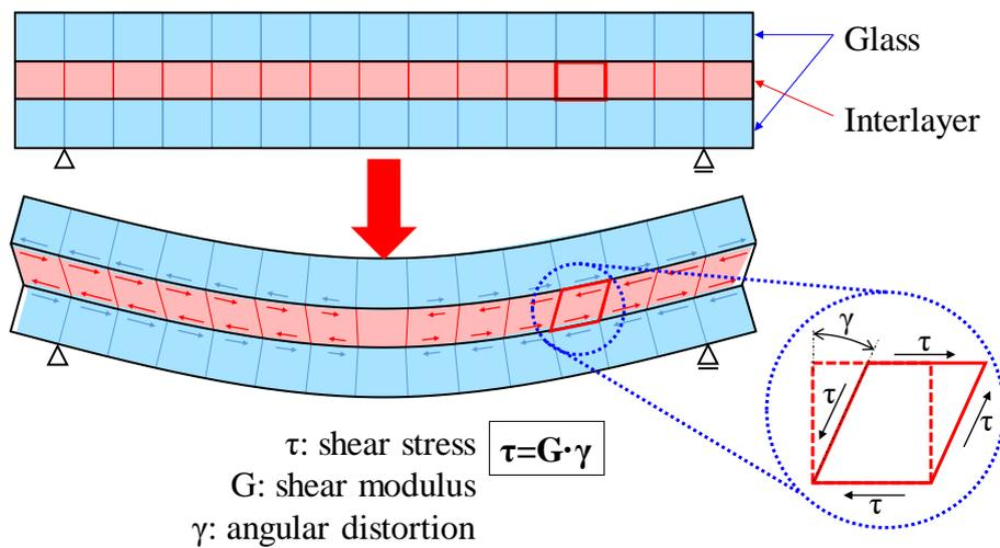
Figure 7. Transfer of shear stress in the interlayer of a laminated glass plate subjected to bending.
