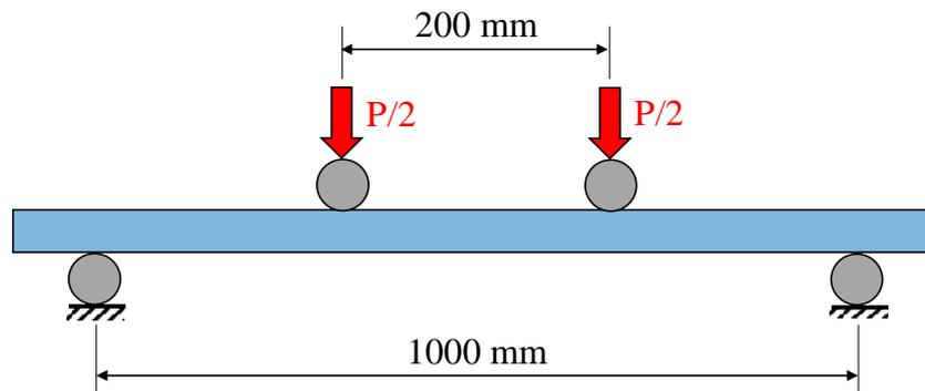
Figure 14. Four-point bending test proposed by the standard ISO 1288-3 [39].
