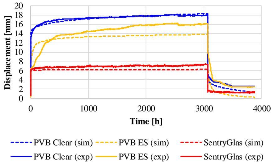
Figure 31. Creep and deflection recovery of three laminated glass plates under long-term loading. Comparison between the experimental results (exp) and the numerical predictions (sim).
