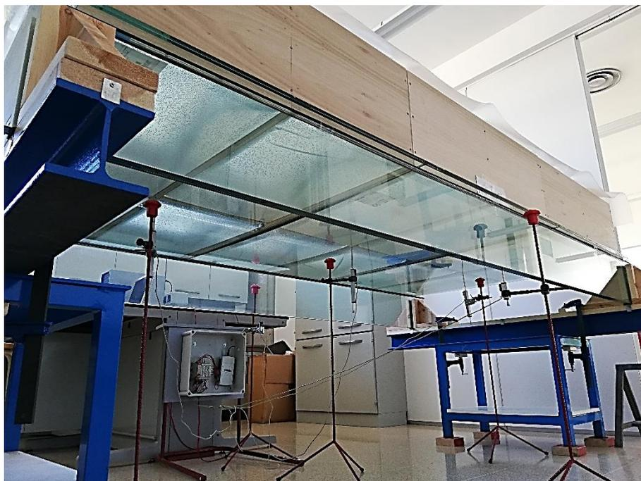
Figure 25. Displacement sensors to measure the vertical deflection at the midspan of the plates and the beams.
