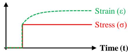
Figure 10. Creep experienced by a viscoelastic material under a constant stress in a stationary test.
