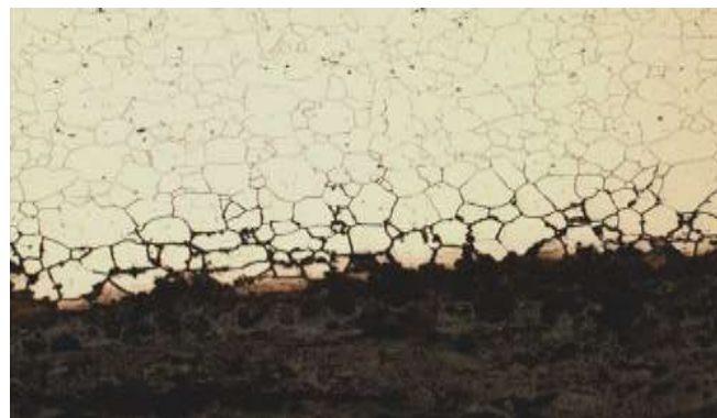
Figure 12. Stainless steel part showing IGA [63]
