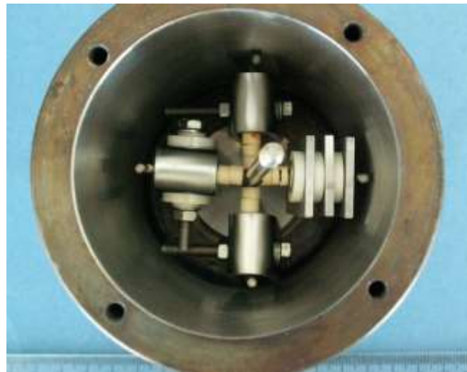
Figure 22. Corrosion coupons assembly to metallic tree inside test crucibles before adding the salt
