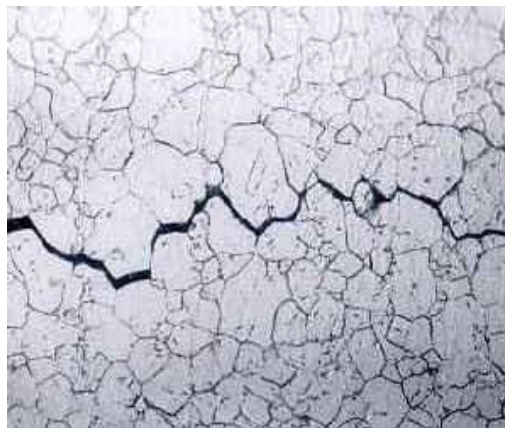
Figure 13. Heat exchanger tube SCC [64]
