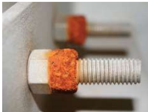
Figure 9. Galvanic corrosion produced in a joint between screw and nut [50]
