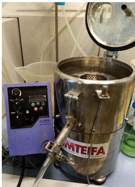
Figure 18. Laboratory scale centrifuge (360 g capacity) from Comteifa used at Farmhispania S.A. to perform filtration studies.
