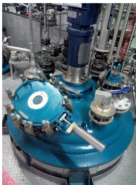
Figure 14. Reactor head picture showing the reactor manway and the auxiliary connections used for the vessel feeding, for the gas venting and for the reflux condenser connection among others.
