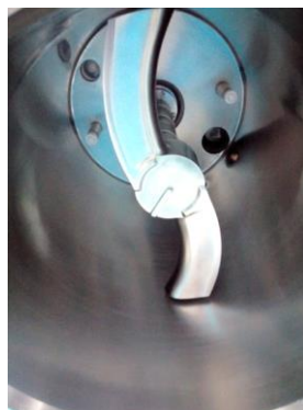
Figure 16. Detail of the stirring arms of an 80 L capacity agitated Nutsche filter property of Farmhispania S.A.
