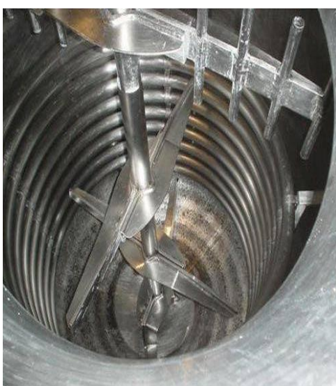
Figure 33. Inside view of a reactor equipped with an internal coil. 34
