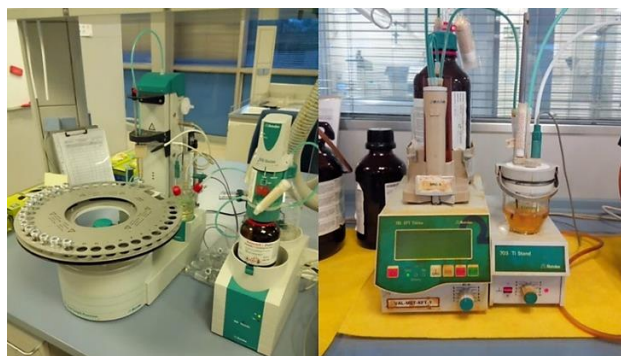
Figure 53. KF oven (left) and volumetric KF (right) both from Metrohm used during the DH0517 process development.
