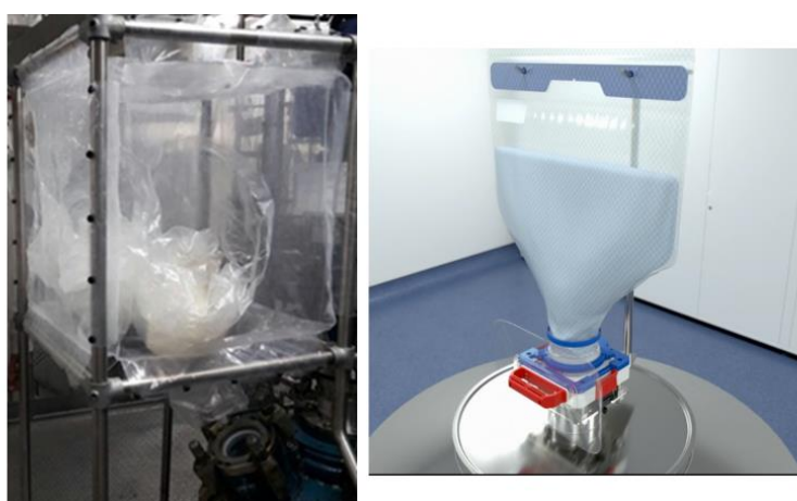
Figure 24. Closed solid addition systems used in Farmhispania S.A. Left: isolator system. Right: scheme of a device from Ezidock Systems. 25
