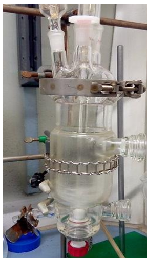
Figure 47. 250 mL reactor used during the reactivity optimization experiments.
