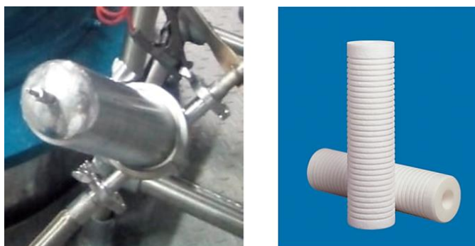
Figure 56. Cuno filters (right) and Cuno filter housing (left) used to perform the microfiltration at industrial scale. 97
