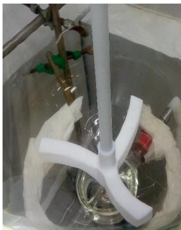
Figure 91. Example of a mechanical stirrer used during the scale-up studies carried out in the laboratory.
