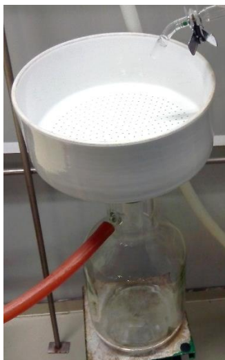
Figure 52. Filtration set-up used during the filtration tests formed by a 5 L Kitasato and a \varnothing=26 cm Büchner funnel.
