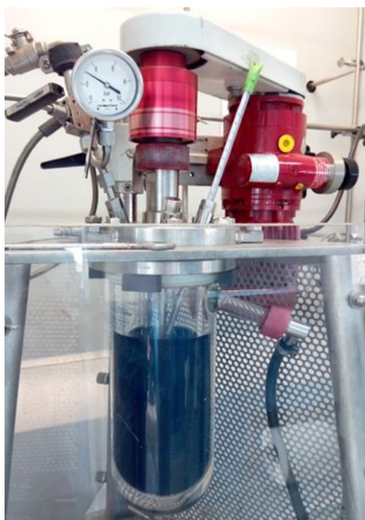
Figure 82. 1.6 L hydrogenator used to perform laboratory gas hydrogenation tests.
