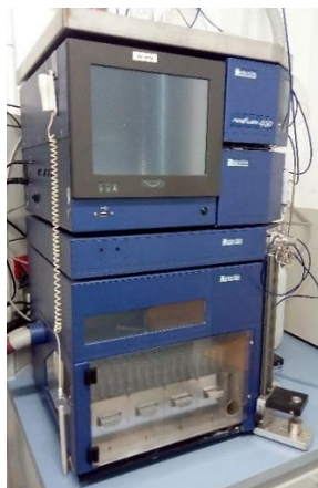
Figure 63. MPLC apparatus Puriflash 450 from Interchim used in Farmhispania S.A.
