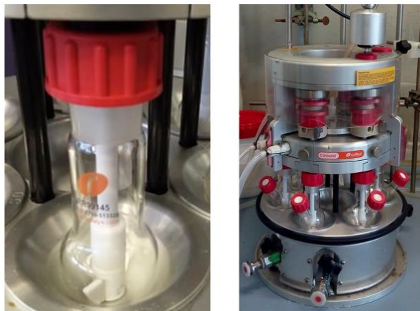
Figure 84. Radleys multi-reactor used to perform the step 2 DoE studies (right). Detail of a Radleys 25 mL reactor provided of mechanical stirring (left).
