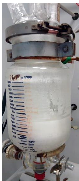
Figure 38. Crusting observed in a 2 L reactor during an evaporative crystallization.
