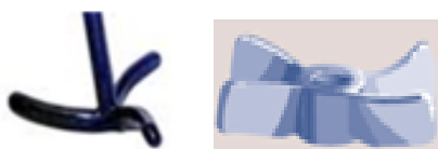
Figure 51. Impeller geometries used for the Dynochem software simulations. Left: retreat curve impeller (RCI). Right: curved blade turbine (CBT)
