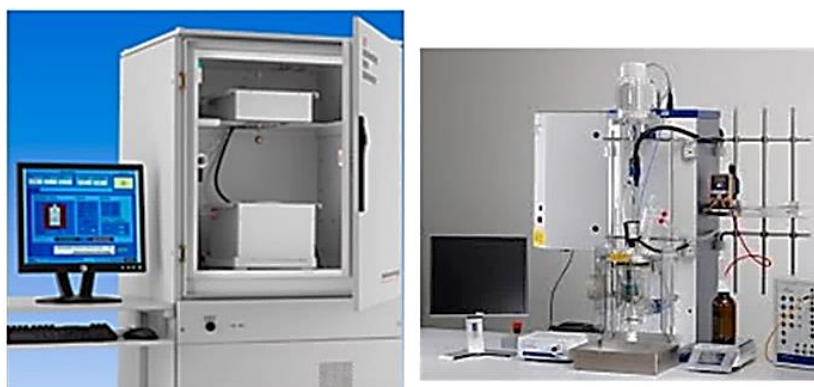
Figure 31. Adiabatic calorimeter from Thermal Hazard Technology (left) and isothermal calorimeter RC-1 from Mettler Toledo (right). Reproduced from Ref 32 with permission of the copyright holder. 33
