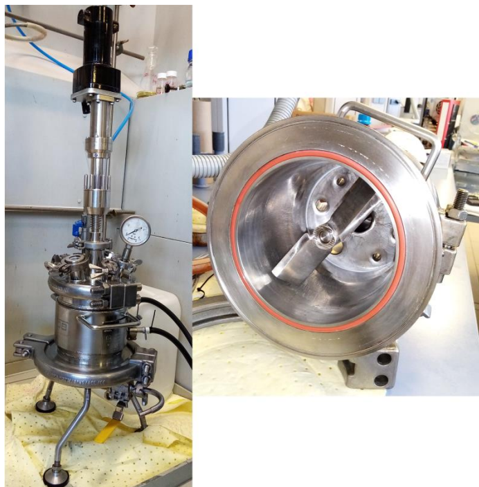
Figure 54. Outside view (right) and inside view (left) of the laboratory scale Nutsche agitated filter used during the laboratory scale tests performed. The filter was provided by Pope Scientific INC.
