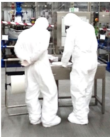
Figure 23. Farmhispania S.A. plant operators wearing a Tychem suite during the manipulation of a hazardous chemical.
