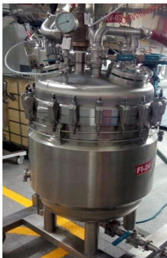
Figure 90. 292 L capacity Nutsche filter used at plant for the FH-4 isolation.
