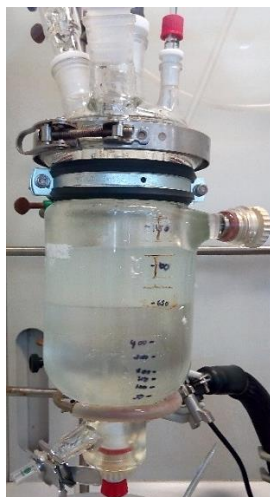
Figure 36. 1 L glass reactor used at Farmhispania S.A. to study a phase separation.
